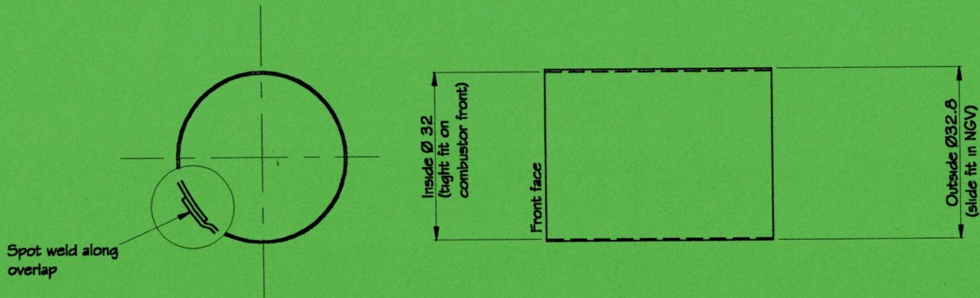
Material: Stainless Steel sheet .4mm thick
