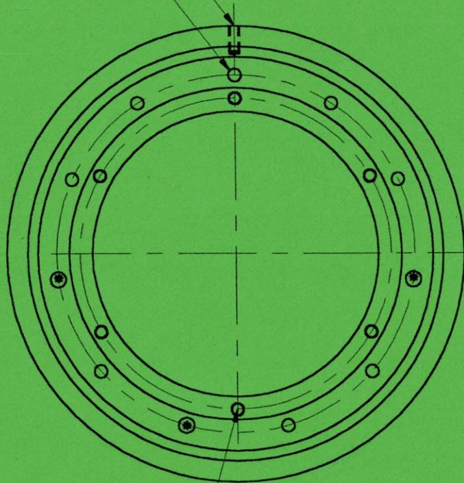
6 Holes Tap M2.5 Equi-spaced on 60 PCD
