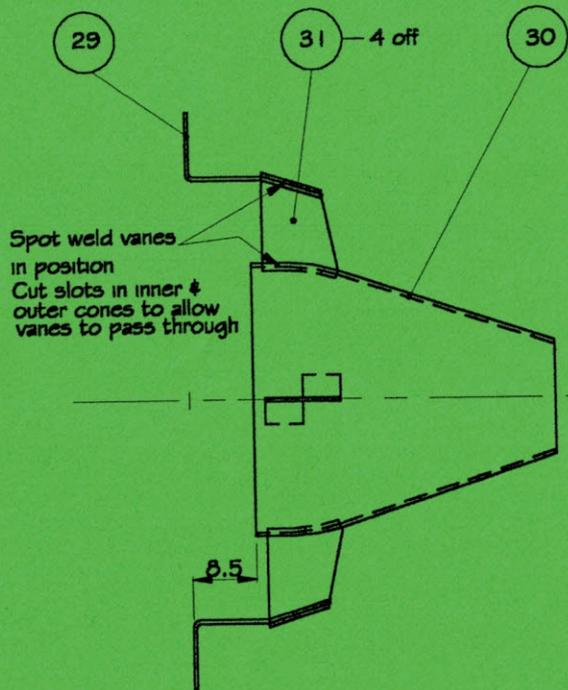
Ensure cone inner and cone outer are concentric.
