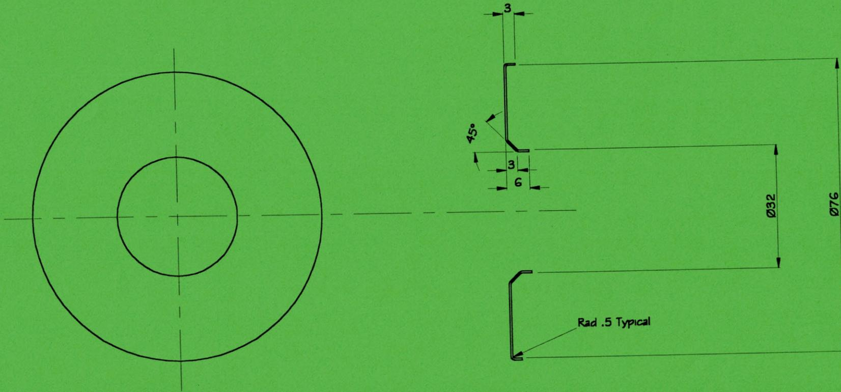
Material: Stainless Steel sheet - .4mm Thick
