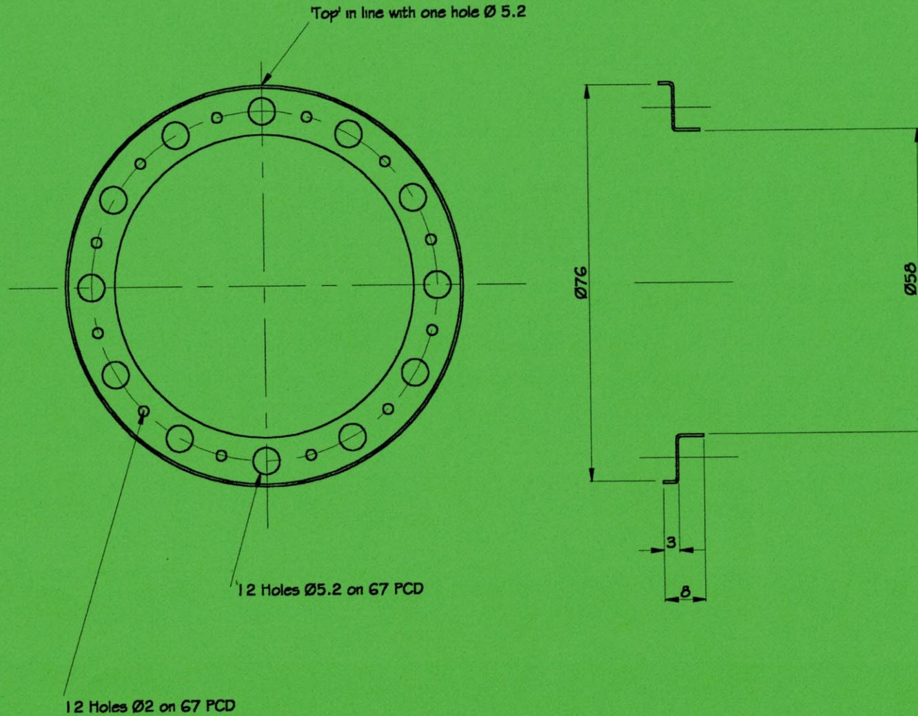
Material: Stainless Steel sheet - .4mm thick
