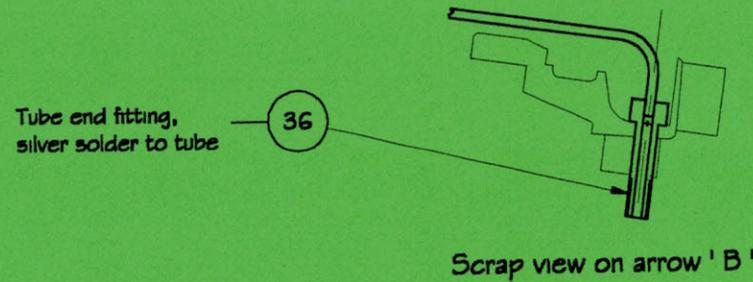
NOTE: Filter and filter cover must be fitted before tube is fitted to diffuser.
