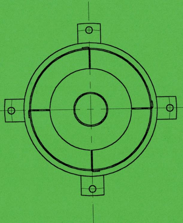
Alternative tangential vanes in 3 positions spot weld in place
