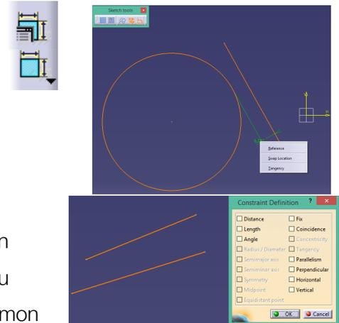
When you have selected one or more feature(s) that can have constraints, the constraints defined in dialogue box tool becomes selectable. This give you a number of options based one the features selected. Once a constraint has been selected, it will preview it (e.g. selecting the perpendicular constraint will preview the lines at their new positions), before applying it when you have clicked ok. Once the constraint is in place, you can edit it by double clicking with MB1.
