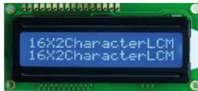
FIGURA 7.2 Display LCD 16 x 2.
