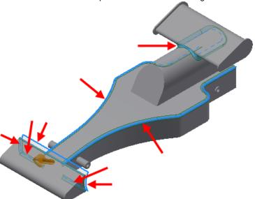
9) Use the Fillet command to place **7 mm** fillets to the four edges as shown.
