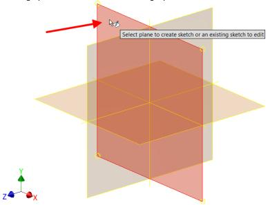
5) Sketch the profile (outline) of the side view of the car body by right-clicking on a blank area in the graphics window and click Create Line on the marking menu, or press the L key or click Sketch tab > Draw panel > Line.
