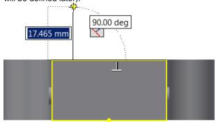
b) While still in the line command, click on the top endpoint of the line and a small gray circle will appear. Click on the small circle, and with the left mouse button pressed down, move the cursor up and to the
