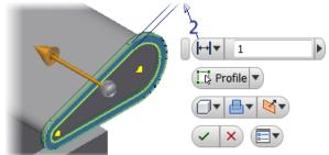
6) Next mirror the side plate to the other side by using the Mirror command on the 3D Model tab > Pattern panel.
