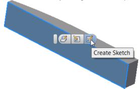
15) Sketch for the area that will be removed, right-click on a blank area in the graphics window and click Create Line on the marking menu and select on the left-vertical line about a quarter of the way up and create a 50 mm line.
