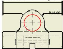
9) There may be times that you want to place additional dimension to clarify the design. To add a dimension either move the cursor so it is outside a drawing view then right-click and click General Dimension from the marking menu or click the Dimension command on the Annotate tab > Dimension panel.
