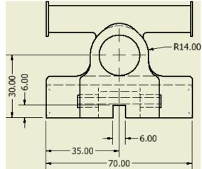
10) Next you add a hole note to document the size of the hole that will contain the CO2 cartridge. Start the Hole and Thread Notes command on the Annotate tab > Feature Notes panel.
