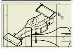
a) Next move the base view (first view placed, which in this exercise is the front view) down and to the left. Notice that the orthographic views (top and side views) will move with it.
