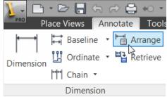
7) Adjust the location of a dimension by moving the cursor over the dimension you want to move until the symbol appears and then click and drag it to a new location. Move the 2.00 aligned dimension in the front view as shown.
