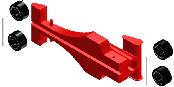
6) Next you assemble the race car using assembly constraints. If you are using Inventor 2013 the first part that you place will be grounded, meaning that it does not move. If you are using Inventor 2014, the first placed component is not automatically grounded. Click and drag on the car body, if it is ground a stick pin symbol will appear. If it is not grounded the part will move. If needed, ground the car body by moving the cursor over
