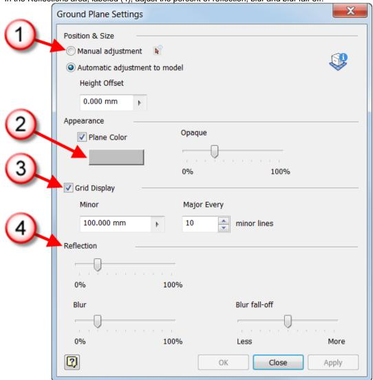
f) Change the size of the ground plane by clicking the Manual adjustment option and click and drag on an edge on the ground plane.
