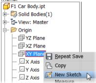
b) The problem is that the sketch is in the middle of the part and you cannot see the sketch. Remove the front section in front of the sketch by clicking the Slice Graphics command on the Status Bar or by
