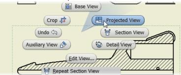
a) Locate the view by clicking a point above and to the left of the cross section view.
