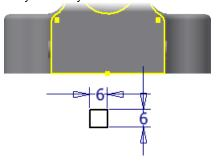
c) Next you constrain the sketch by applying a coincident constraint that will lock two points together. Apply a Coincident sketch constraint by clicking the Sketch tab > Constrain panel > Coincident Constraint.
