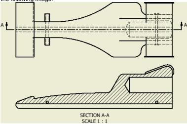
7) To see the cross section view from an angle you create an isometric view by using the Projected View command. To create an isometric view of the cross section view, right-click in the cross section view and click Projected View from the marking menu. You can also access the Projected View command from the
