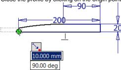
Finish the Line command by right-clicking on a blank area in the graphics window and click OK on the marking menu.
