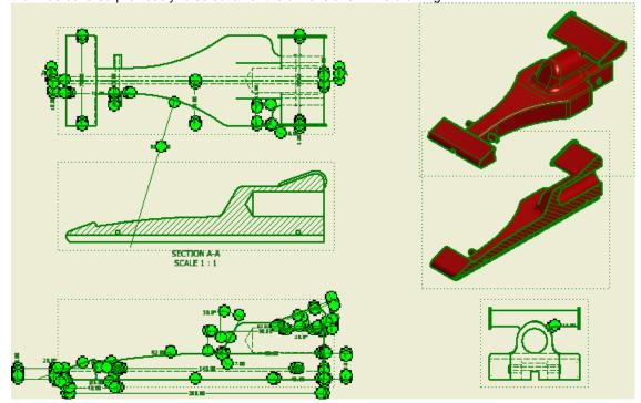
a) Start the Arrange Dimensions command by clicking the Annotate tab > Dimension panel. The dimensions will automatically be arranged based on the current dimension style.
