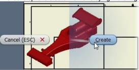
4) Next you move the drawing views to better fit the drawing. Move the cursor over the isometric view until the symbol appears and then click and drag the view to the right of the top view.
