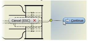
e) Position the section view by clicking a point below the top view. When done your view should resemble the following image.
