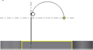
c) Complete the profile by clicking a point on the top horizontal edge so the line is tangent to the arc and perpendicular to the top edge of the sketch.
