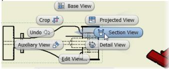
a) If you started the command from the Create panel you need to select the view to section, click inside the top view, if you started the command by right-clicking in the top view the view is already selected.
