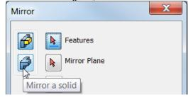
b) Next you select the plane to mirror the body about, move the cursor over the front vertical plane and let the cursor stay still for two seconds and the Select Other toolbar appears, click the drop down arrow and click the second face option (the bottom plane).
