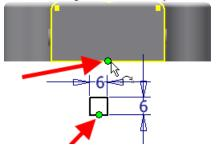
e) Extrude the square profile with the cut operation and the Extents option set to Through All.
