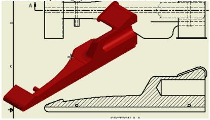
b) Move the isometric view of the cross\_section view so it is below the existing isometric view.
