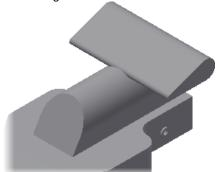
3) Next you create a side plate on the rear wing. Create a sketch on the side plane on the rear wing.
