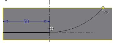
b) Start the dimension command and add a 10 mm linear and 120 mm radius dimension as shown.
