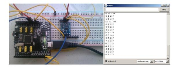
Alternatively, you can set a ±threshold value to detect the tilted position of the module. Replace the Serial.printf function to the if statements written at the last part of the sample sketch.
