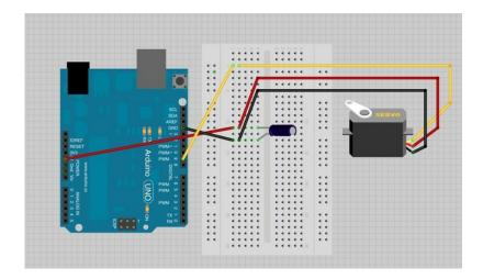
The capacitor acts as a reservoir of electricity for the motor to use, so that when it starts, it takes charge from the capacitor as well as the Arduino supply.
