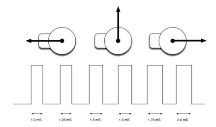
The end points of the servo can vary and many servos only turn through about 170 degrees. You can also buy 'continuous' servos that can rotate through the full 360 degrees.
