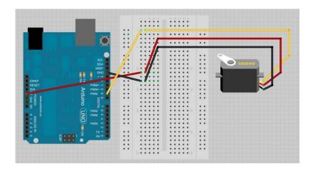
The servo motor has three leads. The color of the leads varies between servo motors, but the red lead is always 5V and GND will either be black or brown. The other lead is the control lead and this is usually orange or yellow. This control lead is connected to digital pin 9.
