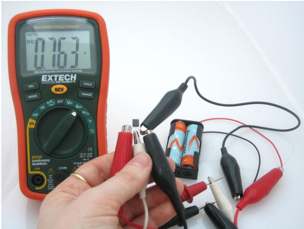
*The sensor is indicating that the temperature is 26.3°C also known as 79.3°F*
