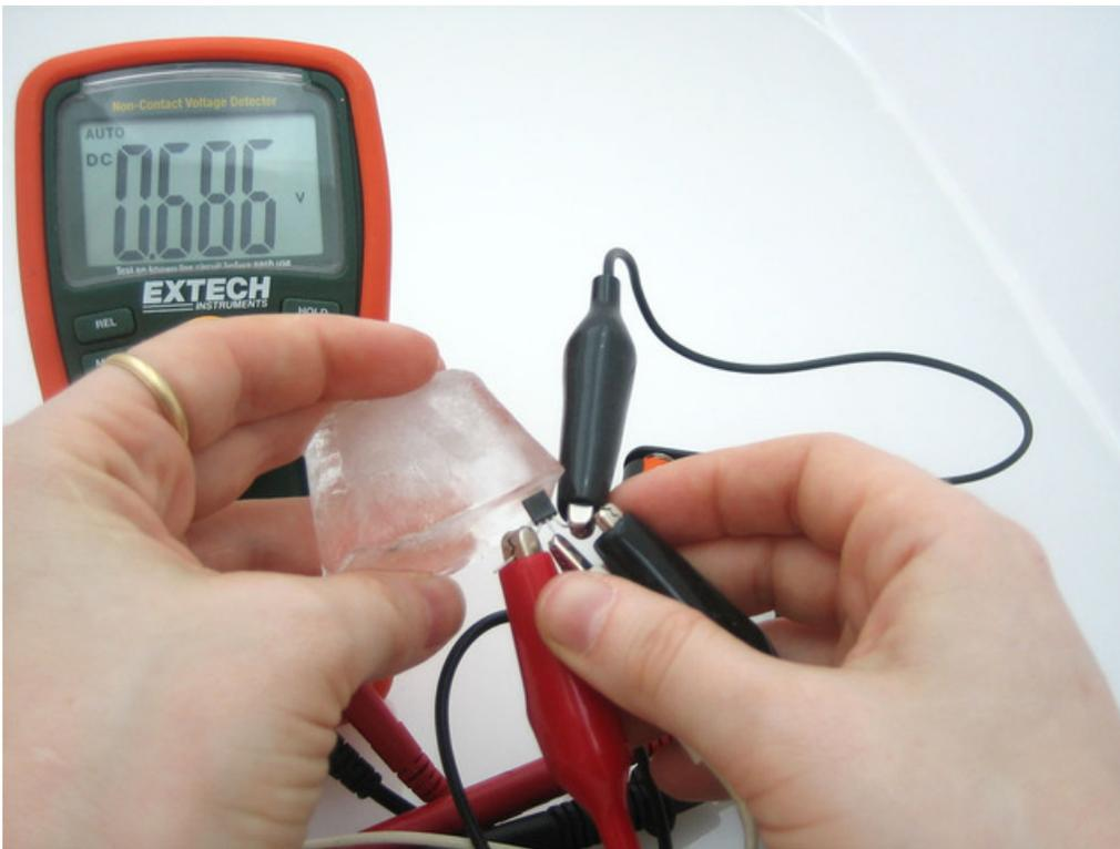
*I pressed an ice-cube against the sensor, to bring the temperature down to 18.6°C / 65.5°F*
