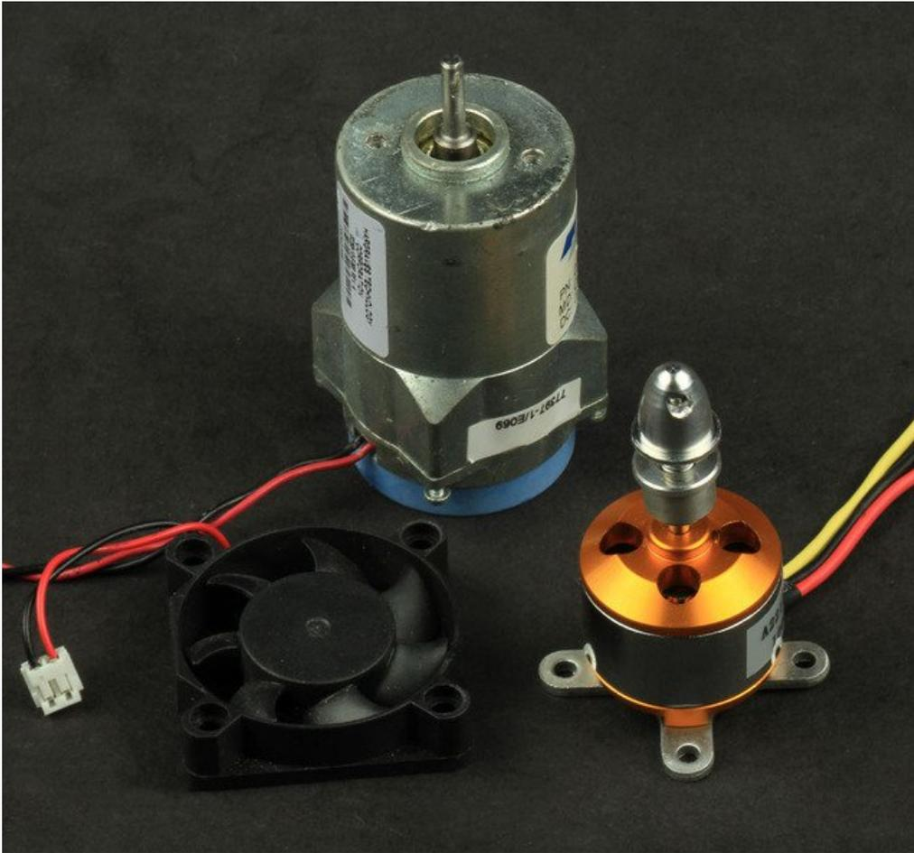
Brushless DC (BLDC) Motors are mechanically simpler than brushed motors. They replace the brushes and associated sparks and noise with electronic commutation to silently switch the current flow to drive the motor. These quiet motors can be found in computer fans and disk drives, as well as in quadcopters, electric vehicles and high-precision servomechanisms.
