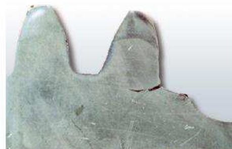
Figure 3. Fatigue Crack in Gear Tooth Root Fillet.
