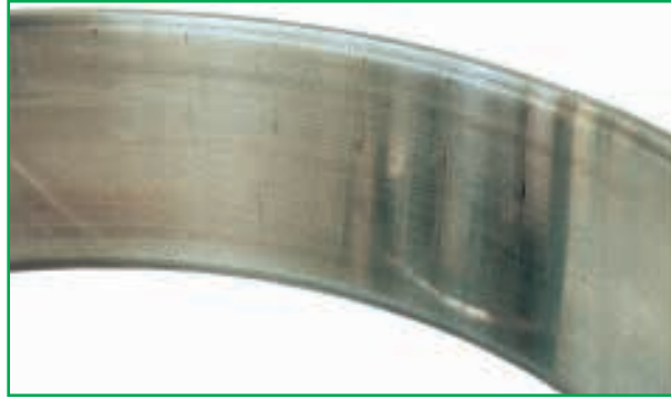
Fig. 24 Part: outer ring of a double-row cylindrical roller bearing Symptom: axial scratches at roller pitch intervals on raceway surface Cause: inclination of inner and outer rings during mounting
