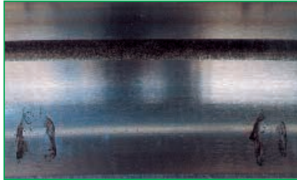
Fig. 6 Part: outer ring of a slewing ring Symptom: rust on raceway surface at ball pitch Cause: moisture condensation during stationary periods
