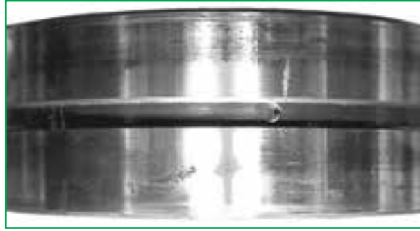
Fig. 18 Highly polished outside surface of outer ring over entire circumference, scratches and indications of fretting corrosion partly visible
