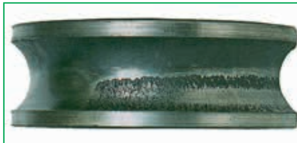
Fig. 20 Oblique running path flaking pattern on inner ring raceway
