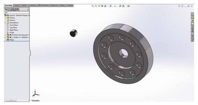
Next activate the Mate tool located in the Assembly tab.
