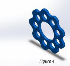
different points. For example you can make a line based on the curve  $y = x^2$  starting from 0 and ending at 10. Using Parametric Curves works the same way as the Explicit but the only difference is that you use two equations to define a curve (an x-component and a y-component). For our purposes we are going to need to use a Parametric Curve because of the two equations needed to define the Rotor.
