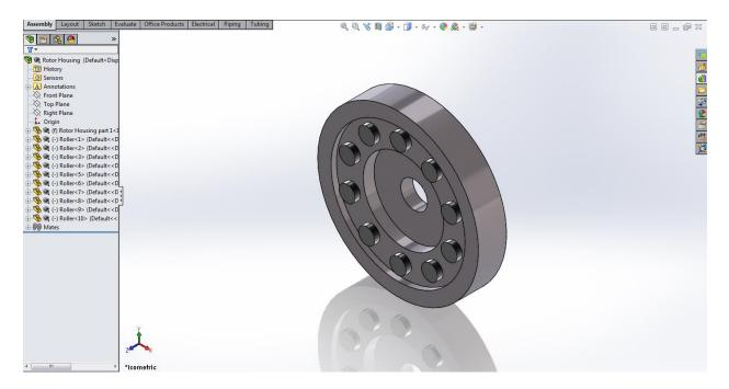
Now it's time to build the Cycloidal Drive assembly. Open a new assembly and insert the Rotor Housing Sub-Assembly we just created into the current assembly.
