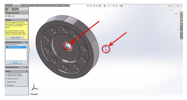
Move your mouse over to the Assembly's origin. Your curser should snap to the assembly origin once you place it near it. Both origins should have merged to show one. Once that happens, click to place the Rotor housing part on the Assembly's origin.
