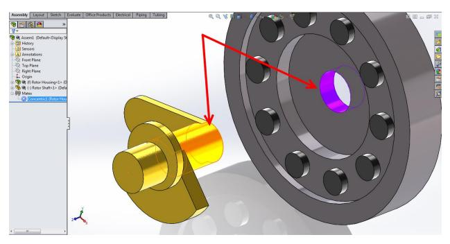
Add a Concentric mate between the Rotor Shaft and Housing using the face shown below.
