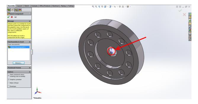
Next click the Insert Components button located in the Assembly tab. Next click Browse in the Insert Components Wizard as we did before and open the Roller part.
