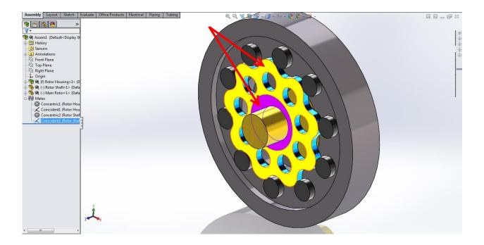
Next we are going to add the two mates that give the Cyclodial Drive its motion. It is very important that these mates are done properly as instructed or else the drive will not function correctly.
