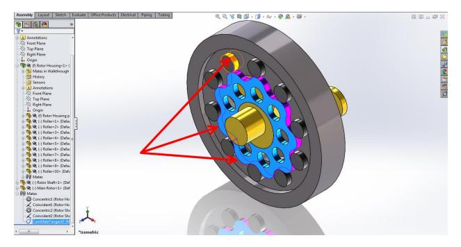
Rebuild the assembly to make sure the mate was applied properly. If a warning appears, you will have to edit the mate and flip the mate direction.
