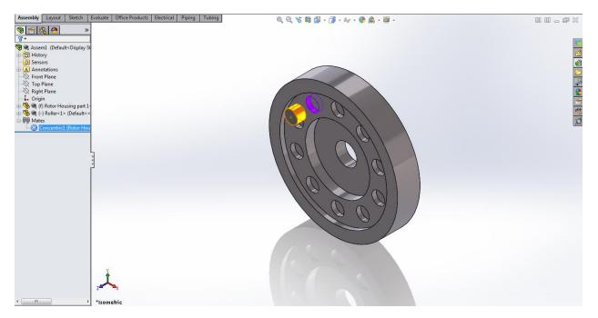
Next create a coincident mate between the back face of the Roller and the face of the hole in the Rotor Housing as shown.
