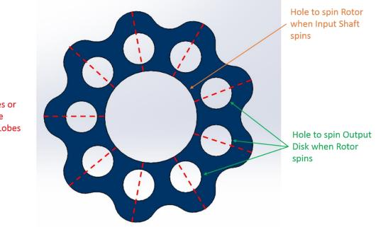
Center of Holes or in line with the center of the Lobes
