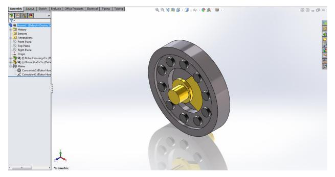
Next insert the Main Rotor part into the assembly.
