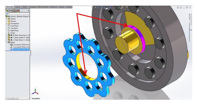
Add a Concentric Mate between the Rotor Shaft and the Main Rotor using the faces shown below.
