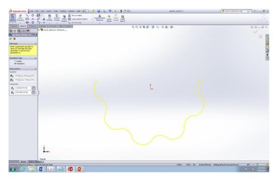
Next draw a centerline that goes through the curve as well as through the Origin and trim the extra parts of the curve with the "Power Trim Tool".
