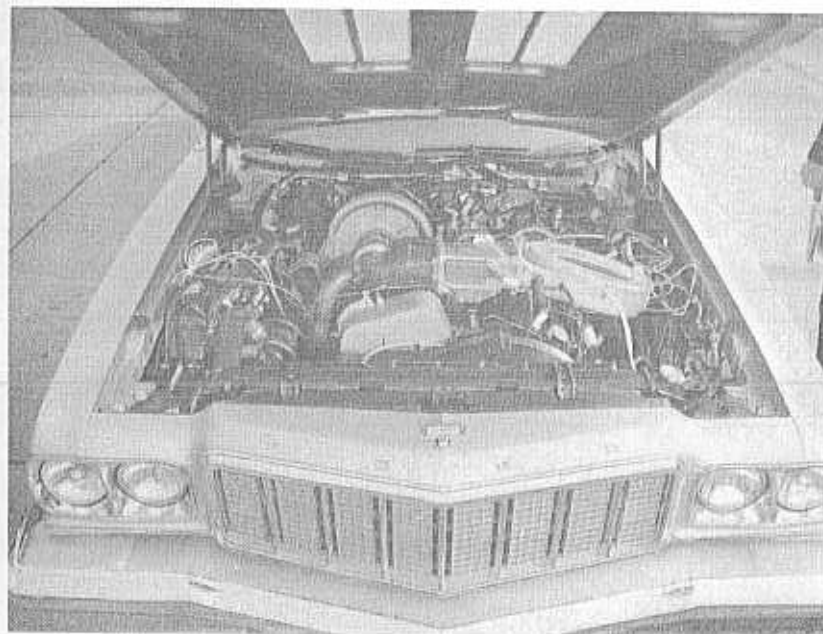
FIG. 12.25. Photograph of the engine compartment of 1973 Ford Torino car with Philips Type 4-215 double-acting Stirling engine installed. (Courtesy Ford Motor Company).
