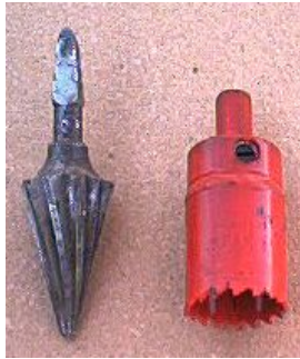
Pipe deburring tool and 1 5/16" hole saw
