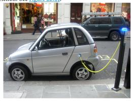
**Figure 20.44** This REVAi, an electric car, gets recharged on a street in London. (credit: Frank Hebbert)
