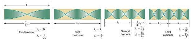
Figure 17.30 The resonant frequencies of a tube open at both ends are shown, including the fundamental and the first three overtones. In all cases the maximum air displacements occur at both ends of the tube, giving it different natural frequencies than a tube closed at one
