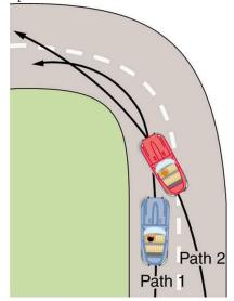
Figure 6.32 Two paths around a race track curve are shown. Race car drivers will take the inside path (called cutting the corner) whenever possible because it allows them to take the curve at the highest speed.
