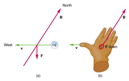
Figure 22.18 A positively charged object moving due west in a region where the Earth's magnetic field is due north experiences a force that is straight down as shown. A negative charge moving in the same direction would feel a force straight up.
