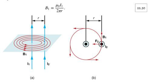
Figure 22.42 (a) The magnetic field produced by a long straight conductor is perpendicular to a parallel conductor, as indicated by RHR-2. (b) A view from above of the two wires shown in (a), with one magnetic field line shown for each wire. RHR-1 shows that the force between the parallel conductors is attractive when the currents are in the same direction. A similar analysis shows that the force is repulsive between currents in opposite directions.
