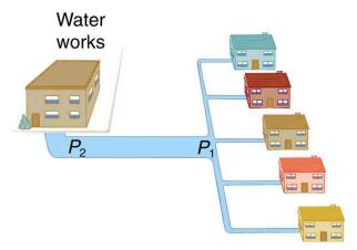
Figure 12.15 During times of heavy use, there is a significant pressure drop in a water main, and  $P_1$  supplied to users is significantly less than  $P_2$  created at the water works. If the flow is very small, then the pressure drop is negligible, and  $P_2 \approx P_1$ .
