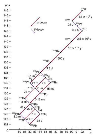
Figure 31.16 The decay series produced by <sup>238</sup> U, the most common uranium isotope. Nuclides are graphed in the same manner as in the chart of nuclides. The type of decay for each member of the series is shown, as well as the half-lives. Note that some nuclides decay by more than one mode. You can see why radium and polonium are found in uranium ore. A stable isotope of lead is the end product of the series.
