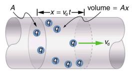
Figure 20.7 All the charges in the shaded volume of this wire move out in a time t, having a drift velocity of magnitude  $v_{\rm d}=x/t$ . See text for further discussion.
