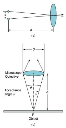
Figure 27.30 (a) Two points separated by at distance *x* and a positioned a distance *d* away from the objective. (credit: Infopro, Wikimedia Commons) (b) Terms and symbols used in discussion of resolving power for a lens and an object at point P. (credit: Infopro, Wikimedia Commons)
