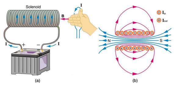
Figure 22.40 (a) Because of its shape, the field inside a solenoid of length *l* is remarkably uniform in magnitude and direction, as indicated by the straight and uniformly spaced field lines. The field outside the coils is nearly zero. (b) This cutaway shows the magnetic field generated by the current in the solenoid.
