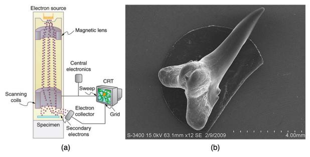
Figure 29.22 Schematic of a scanning electron microscope (SEM) (a) used to observe small details, such as those seen in this image of a tooth of a *Himipristis*, a type of shark (b). (credit: Dallas Krentzel, Flickr)
