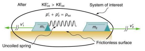
Figure 8.10 An air track is nearly frictionless, so that momentum is conserved. Motion is one-dimensional. In this collision, examined in <a href="Example 8.6">Example 8.6</a>, the potential energy of a compressed spring is released during the collision and is converted to internal kinetic energy.
