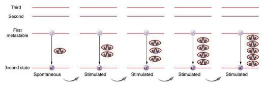
Figure 30.37 One atom in the metastable state spontaneously decays to a lower level, producing a photon that goes on to stimulate another atom to de-excite. The second photon has exactly the same energy and wavelength as the first and is in phase with it. Both go on to stimulate the emission of other photons. A population inversion is necessary for there to be a net production rather than a net absorption of the photons.
