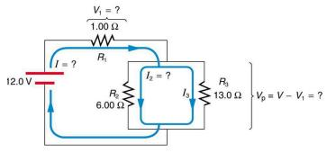
Figure 21.6 These three resistors are connected to a voltage source so that  $R_2$  and  $R_3$  are in parallel with one another and that combination is in series with  $R_1$ .
