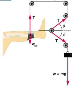
**Figure 4.29** A leg is suspended by a traction system in which wires are used to transmit forces. Frictionless pulleys change the direction of the force *T* without changing its magnitude.
