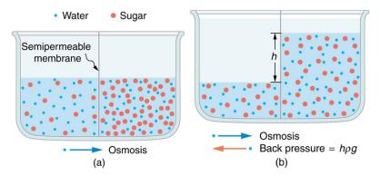
Figure 12.23 (a) Two sugar-water solutions of different concentrations, separated by a semipermeable membrane that passes water but not sugar. Osmosis will be to the right, since water is less concentrated there. (b) The fluid level rises until the back pressure  $\rho gh$  equals the relative osmotic pressure; then, the net transfer of water is zero.
