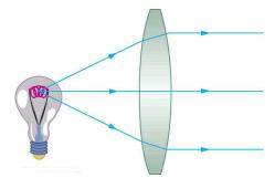
Figure 25.30 A small light source, like a light bulb filament, placed at the focal point of a convex lens, results in parallel rays of light emerging from the other side. The paths are exactly the reverse of those shown in Figure 25.27. This technique is used in lighthouses and sometimes in traffic lights to produce a directional beam of light from a source that emits light in all directions.
