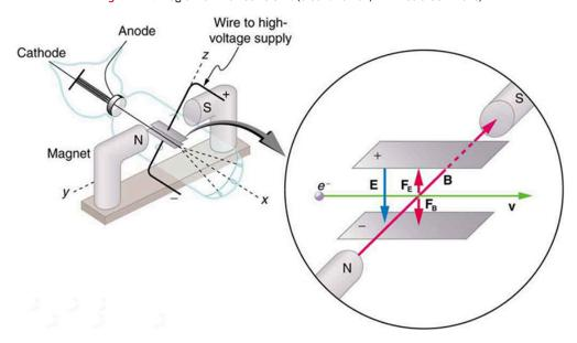
Figure 30.7 This schematic shows the electron beam in a CRT passing through crossed electric and magnetic fields and causing phosphor to glow when striking the end of the tube.
