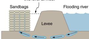
Figure 11.40 Because the river level is very high, it has started to leak under the levee. Sandbags are placed around the leak, and the water held by them rises until it is the same level as the river, at which point the water there stops rising.
