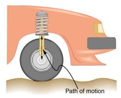
Figure 23.51 The forced but damped motion of the wheel on the car spring is analogous to an *RLC* series AC circuit. The shock absorber damps the motion and dissipates energy, analogous to the resistance in an *RLC* circuit. The mass and spring determine the resonant frequency.
