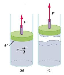
Figure 11.35 (a) When the piston is raised, it stretches the liquid slightly, putting it under tension and creating a negative absolute pressure P = -F/A. (b) The liquid eventually separates, giving an experimental limit to negative pressure in this liquid.
