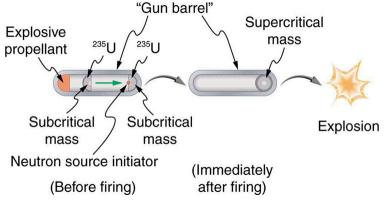
Figure 32.27 A gun-type fission bomb for <sup>235</sup>U utilizes two subcritical masses forced together by explosive charges inside a cannon barrel. The energy yield depends on the amount of uranium and the time it can be held together before it disassembles itself.
