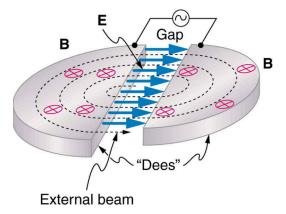
Figure 33.8 Cyclotrons use a magnetic field to cause particles to move in circular orbits. As the particles pass between the plates of the Ds, the voltage across the gap is oscillated to accelerate them twice in each orbit.
