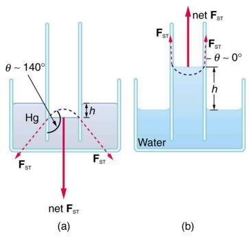
Figure 11.33 (a) Mercury is suppressed in a glass tube because its contact angle is greater than 90°. Surface tension exerts a downward force as it flattens the mercury, suppressing it in the tube. The dashed line shows the shape the mercury surface would have without the flattening effect of surface tension. (b) Water is raised in a glass tube because its contact angle is nearly 0°. Surface tension therefore exerts an upward force when it flattens the surface to reduce its area.
