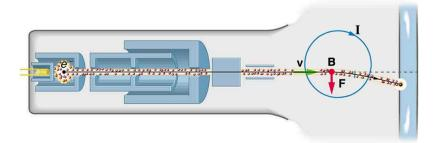
Figure 22.44 The cathode ray tube (CRT) is so named because rays of electrons originate at the cathode in the electron gun. Magnetic coils are used to steer the beam in many CRTs. In this case, the beam is moved down. Another pair of horizontal coils would steer the beam horizontally.
