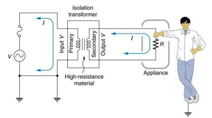
Figure 23.38 An isolation transformer puts a large resistance between the original voltage source and the device, preventing a complete circuit between them.
