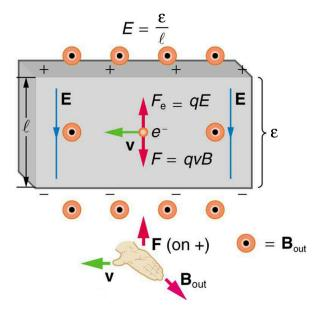
Figure 22.28 The Hall emf  $\varepsilon$  produces an electric force that balances the magnetic force on the moving charges. The magnetic force produces charge separation, which builds up until it is balanced by the electric force, an equilibrium that is quickly reached.
