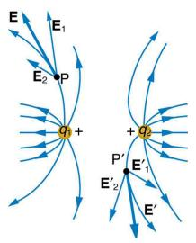
Figure 18.25 Two positive point charges  $q_1$  and  $q_2$  produce the resultant electric field shown. The field is calculated at representative points and then smooth field lines drawn following the rules outlined in the text.
