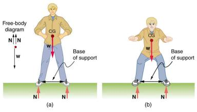
Figure 9.16 (a) The center of gravity of an adult is above the hip joints (one of the main pivots in the body) and lies between two narrowly-
