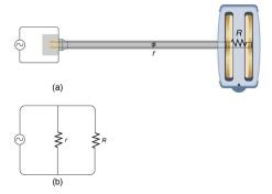
Figure 20.21 A short circuit is an undesired low-resistance path across a voltage source. (a) Worn insulation on the wires of a toaster allow them to come into contact with a low resistance r. Since  $P = V^2/r$ , thermal power is created so rapidly that the cord melts or burns. (b) A schematic of the short circuit.
