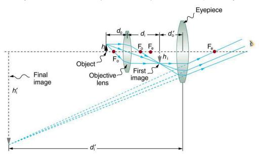
Figure 26.16 A compound microscope composed of two lenses, an objective and an eyepiece. The objective forms a case 1 image that is larger than the object. This first image is the object for the eyepiece. The eyepiece forms a case 2 final image that is further magnified.
