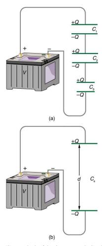
Figure 19.20 (a) Capacitors connected in series. The magnitude of the charge on each plate is Q. (b) An equivalent capacitor has a larger plate separation d. Series connections produce a total capacitance that is less than that of any of the individual capacitors.
