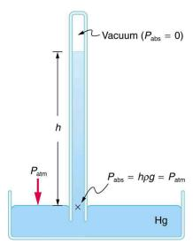
Figure 11.17 A mercury barometer measures atmospheric pressure. The pressure due to the mercury's weight,  $h\rho g$ , equals atmospheric pressure. The atmosphere is able to force mercury in the tube to a height h because the pressure above the mercury is zero.
