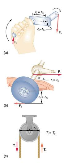
Figure 9.24 (a) A crank is a type of lever that can be rotated 360° about its pivot. Cranks are usually designed to have a large MA. (b) A simplified automobile axle drives a wheel, which has a much larger diameter than the axle. The MA is less than 1. (c) An ordinary pulley is used to lift a heavy load. The pulley changes the direction of the force T exerted by the cord without changing its magnitude. Hence, this machine has an MA of 1.
