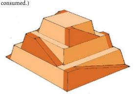
Figure 7.44 Ancient pyramids were probably constructed using ramps as simple machines. (credit: Franck Monnier, Wikimedia Commons)
