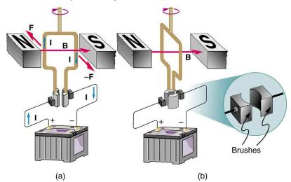
Figure 22.36 (a) As the angular momentum of the coil carries it through  $\theta = 0$ , the brushes reverse the current to keep the torque clockwise. (b) The coil will rotate continuously in the clockwise direction, with the current reversing each half revolution to maintain the clockwise torque.
