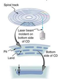
Figure 30.42 A CD has digital information stored in the form of laser-created pits on its surface. These in turn can be read by detecting the laser light scattered from the pit. Large information capacity is possible because of the precision of the laser. Shorter-wavelength lasers enable greater storage capacity.
