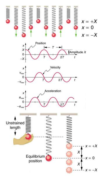
Figure 16.12 Graphs of x(t), v(t), and a(t) versus t for the motion of an object on a spring. The net force on the object can be described by Hooke's law, and so the object undergoes simple harmonic motion. Note that the initial position has the vertical displacement at its maximum value X; v is initially zero and then negative as the object moves down; and the initial acceleration is negative, back toward the equilibrium position and becomes zero at that point.
