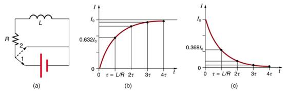
Figure 23.44 (a) An *RL* circuit with a switch to turn current on and off. When in position 1, the battery, resistor, and inductor are in series and a current is established. In position 2, the battery is removed and the current eventually stops because of energy loss in the resistor. (b) A graph of current growth versus time when the switch is moved to position 1. (c) A graph of current decay when the switch is moved to position 2.
