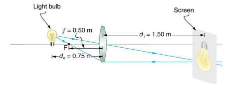
Figure 25.35 A light bulb placed 0.750 m from a lens having a 0.500 m focal length produces a real image on a poster board as discussed in the example above. Ray tracing predicts the image location and size.
