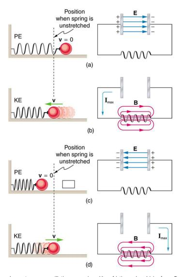
Figure 23.52 An *LC* circuit is analogous to a mass oscillating on a spring with no friction and no driving force. Energy moves back and forth between the inductor and capacitor, just as it moves from kinetic to potential in the mass-spring system.
