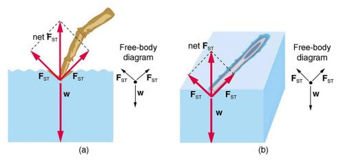
Figure 11.27 Surface tension supporting the weight of an insect and an iron needle, both of which rest on the surface without penetrating it. They are not floating; rather, they are supported by the surface of the liquid. (a) An insect leg dents the water surface.  $F_{ST}$  is a restoring force (surface tension) parallel to the surface. (b) An iron needle similarly dents a water surface until the restoring force (surface tension) grows to equal its weight.
