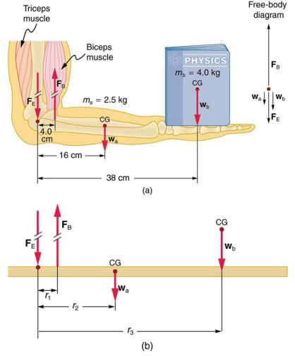
Figure 9.26 (a) The figure shows the forearm of a person holding a book. The biceps exert a force  $\mathbf{F}_B$  to support the weight of the forearm and the book. The triceps are assumed to be relaxed. (b) Here, you can view an approximately equivalent mechanical system with the pivot at the elbow joint as seen in Example 9.4.
