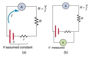
Figure 21.36 Two methods for measuring resistance with standard meters. (a) Assuming a known voltage for the source, an ammeter measures current, and resistance is calculated as  $R = \frac{V}{I}$ . (b) Since the terminal voltage V varies with current, it is better to measure it. V is most accurately known when I is small, but I itself is most accurately known when it is large.
