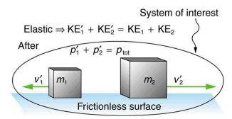
Figure 8.6 An elastic one-dimensional two-object collision. Momentum and internal kinetic energy are conserved.
