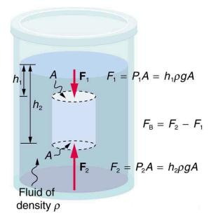
Figure 11.19 Pressure due to the weight of a fluid increases with depth since  $P = h\rho g$ . This pressure and associated upward force on the bottom of the cylinder are greater than the downward force on the top of the cylinder. Their difference is the buoyant force  $\mathbf{F}_{\mathrm{B}}$ . (Horizontal forces cancel.)
