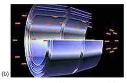
Figure 26.26 (a) The Australia Telescope Compact Array at Narrabri (500 km NW of Sydney). (credit: Ian Bailey) (b) The focusing of x rays on the Chandra Observatory, a satellite orbiting earth. X rays ricochet off 4 pairs of mirrors forming a barrelled pathway leading to the focus point. (credit: NASA)
