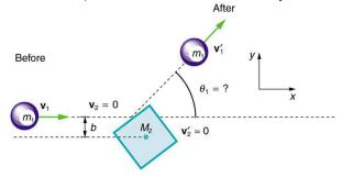
Figure 8.16 A small object approaches a collision with a much more massive cube, after which its velocity has the direction  $\theta_1$ . The angles at which the small object can be scattered are determined by the shape of the object it strikes and the impact parameter b.
