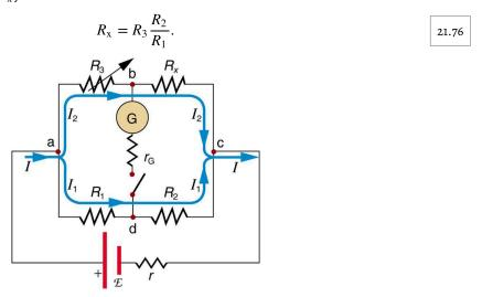
Figure 21.37 The Wheatstone bridge is used to calculate unknown resistances. The variable resistance  $R_3$  is adjusted until the galvanometer reads zero with the switch closed. This simplifies the circuit, allowing  $R_x$  to be calculated based on the IR drops as discussed in the text.
