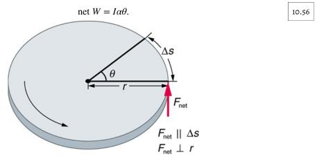
Figure 10.15 The net force on this disk is kept perpendicular to its radius as the force causes the disk to rotate. The net work done is thus  $(\text{net } F)\Delta s$ . The net work goes into rotational kinetic energy.
