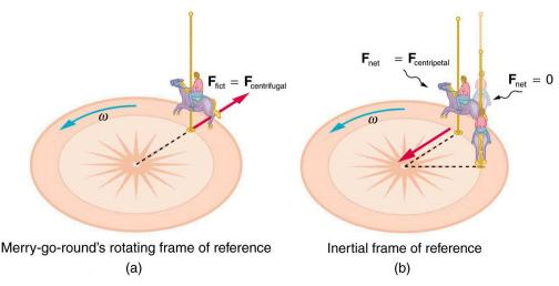
Figure 6.16 (a) A rider on a merry-go-round feels as if he is being thrown off. This fictitious force is called the centrifugal force—it explains the rider's motion in the rotating frame of reference. (b) In an inertial frame of reference and according to Newton's laws, it is his inertia that carries him off and not a real force (the unshaded rider has  $F_{\rm net}=0$  and heads in a straight line). A real force,  $F_{\rm centripetal}$ , is needed to cause a circular path.
