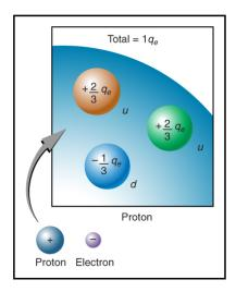
Figure 18.7 Artist's conception of fractional quark charges inside a proton. A group of three quark charges add up to the single positive charge on the proton:  $-\frac{1}{3}q_e + \frac{2}{3}q_e + \frac{2}{3}q_e = +1q_e$ .
