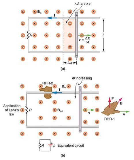
Figure 23.11 (a) A motional emf =  $B\ell\nu$  is induced between the rails when this rod moves to the right in the uniform magnetic field. The magnetic field B is into the page, perpendicular to the moving rod and rails and, hence, to the area enclosed by them. (b) Lenz's law gives the directions of the induced field and current, and the polarity of the induced emf. Since the flux is increasing, the induced field is in the
