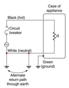
Figure 23.32 The three-wire system connects the neutral wire to the earth at the voltage source and user location, forcing it to be at zero volts and supplying an alternative return path for the current through the earth. Also grounded to zero volts is the case of the appliance. A
