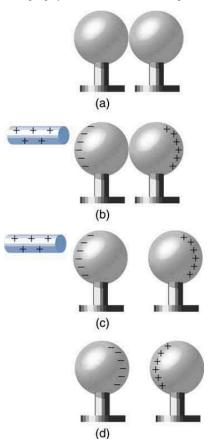
Figure 18.13 Charging by induction. (a) Two uncharged or neutral metal spheres are in contact with each other but insulated from the rest of the world. (b) A positively charged glass rod is brought near the sphere on the left, attracting negative charge and leaving the other sphere positively charged. (c) The spheres are separated before the rod is removed, thus separating negative and positive charge. (d) The
