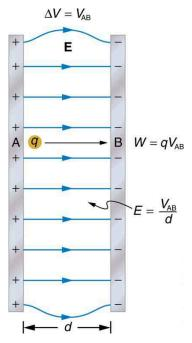
Figure 19.5 The relationship between V and E for parallel conducting plates is E = V/d. (Note that  $\Delta V = V_{AB}$  in magnitude. For a charge that is moved from plate A at higher potential to plate B at lower potential, a minus sign needs to be included as follows:  $-\Delta V = V_{A} - V_{B} = V_{AB}$ . See the text for details.)
