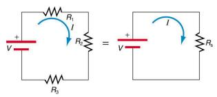
Figure 21.3 Three resistors connected in series to a battery (left) and the equivalent single or series resistance (right).
