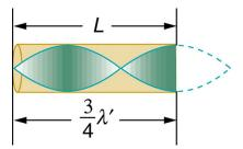
Figure 17.27 Another resonance for a tube closed at one end. This has maximum air displacements at the open end, and none at the closed end. The wavelength is shorter, with three-fourths  $\lambda'$  equaling the length of the tube, so that  $\lambda' = 4L/3$ . This higher-frequency vibration is the first overtone.
