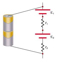
Figure 21.15 A series connection of two voltage sources. The emfs (each labeled with a script E) and internal resistances add, giving a total emf of emf<sub>1</sub> + emf<sub>2</sub> and a total internal resistance of  $r_1 + r_2$ .
