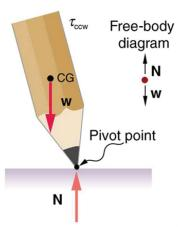
Figure 9.14 If the pencil is displaced even slightly, a torque is created by its weight that is in the same direction as the displacement, causing the displacement to increase.
