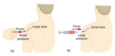
Figure 11.6 (a) While the person being poked with the finger might be irritated, the force has little lasting effect. (b) In contrast, the same force applied to an area the size of the sharp end of a needle is great enough to break the skin.
