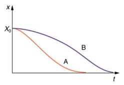
Figure 16.23 Displacement versus time for a critically damped harmonic oscillator (A) and an overdamped harmonic oscillator (B). The critically damped oscillator returns to equilibrium at X = 0 in the smallest time possible without overshooting.
