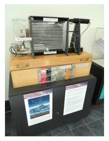
Figure 19.6 A spark chamber is used to trace the paths of high-energy particles. Ionization created by the particles as they pass through the gas between the plates allows a spark to jump. The sparks are perpendicular to the plates, following electric field lines between them. The potential difference between adjacent plates is not high enough to cause sparks without the ionization produced by particles from accelerator experiments (or cosmic rays). (credit: Daderot, Wikimedia Commons)
