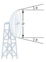
Figure 27.29 The beam produced by this microwave transmission antenna will spread out at a minimum angle  $\theta = 1.22 \ \lambda/D$  due to diffraction. It is impossible to produce a near-parallel beam, because the beam has a limited diameter.
