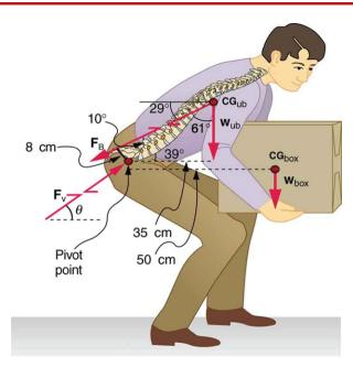
Figure 9.29 This figure shows that large forces are exerted by the back muscles and experienced in the vertebrae when a person lifts with their back, since these muscles have small effective perpendicular lever arms. The data shown here are analyzed in the preceding example, Example 9.5.
