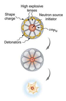
Figure 32.28 An implosion created by high explosives compresses a sphere of <sup>239</sup>Pu into a critical mass. The superior fissionability of plutonium has made it the universal bomb material.
