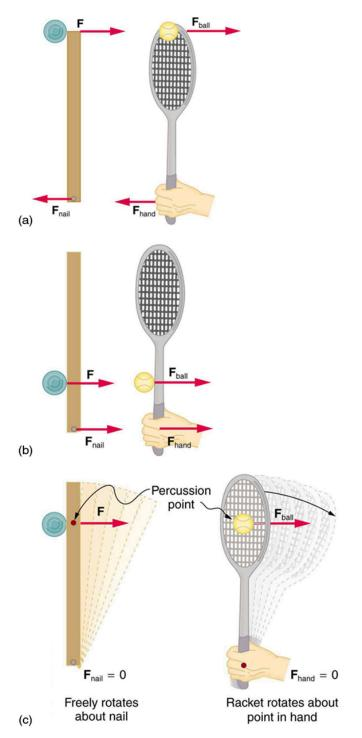
Figure 10.27 A disk hitting a stick is compared to a tennis ball being hit by a racquet. (a) When the ball strikes the racquet near the end, a backward force is exerted on the hand. (b) When the racquet is struck much farther down, a forward force is exerted on the hand. (c) When the racquet is struck at the percussion point, no force is delivered to the hand.
