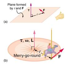
Figure 10.29 In figure (a), the torque is perpendicular to the plane formed by r and  $\mathbf{F}$  and is the direction your right thumb would point to if you curled your fingers in the direction of  $\mathbf{F}$ . Figure (b) shows that the direction of the torque is the same as that of the angular momentum
