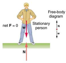
Figure 9.2 This motionless person is in static equilibrium. The forces acting on him add up to zero. Both forces are vertical in this case.
