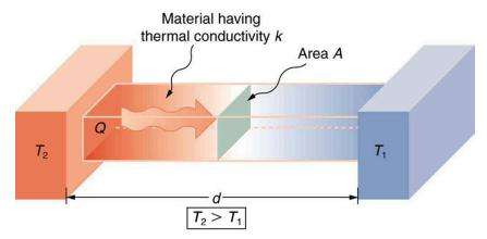
Figure 14.15 Heat conduction occurs through any material, represented here by a rectangular bar, whether window glass or walrus blubber. The temperature of the material is  $T_2$  on the left and  $T_1$  on the right, where  $T_2$  is greater than  $T_1$ . The rate of heat transfer by conduction is directly proportional to the surface area A, the temperature difference  $T_2 - T_1$ , and the substance's conductivity k. The rate of heat transfer is inversely proportional to the thickness d.
