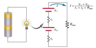
Figure 21.18 This schematic represents a flashlight with two cells (voltage sources) and a single bulb (load resistance) in series. The current that flows is  $I = \frac{(\text{emf}_1 + \text{emf}_2)}{r_1 + r_2 + R_{\text{load}}}$ . (Note that each emf is represented by script E in the figure.)
