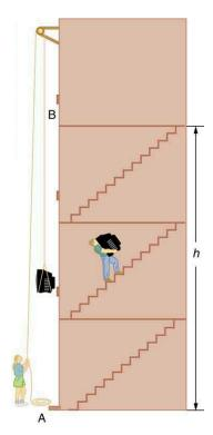
Figure 7.6 The change in gravitational potential energy ( $\Delta PE_g$ ) between points A and B is independent of the path.  $\Delta PE_g = mgh$  for any path between the two points. Gravity is one of a small class of forces where the work done by or against the force depends only on the starting and ending points, not on the path between them.
