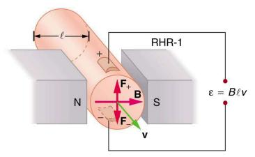
Figure 22.29 The Hall effect can be used to measure fluid flow in any fluid having free charges, such as blood. The Hall emf  $\varepsilon$  is measured across the tube perpendicular to the applied magnetic field and is proportional to the average velocity v.
