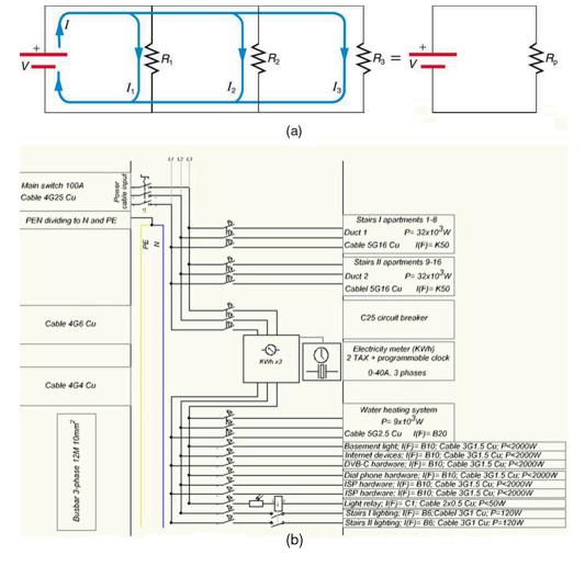
Figure 21.4 (a) Three resistors connected in parallel to a battery and the equivalent single or parallel resistance. (b) Electrical power setup in a house. (credit: Dmitry G, Wikimedia Commons)
