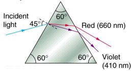
Figure 25.57 This prism will disperse the white light into a rainbow of colors. The incident angle is  $45.0^{\circ}$ , and the angles at which the red and violet light emerge are  $\theta_R$  and  $\theta_V$ .
