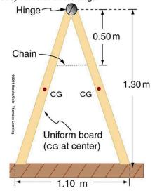
**Figure 9.34** A sandwich board advertising sign demonstrates tension.
