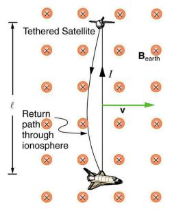
Figure 23.12 Motional emf as electrical power conversion for the space shuttle is the motivation for the Tethered Satellite experiment. A 5 kV emf was predicted to be induced in the 20 km long tether while moving at orbital speed in the Earth's magnetic field. The circuit is completed by a return path through the stationary ionosphere.
