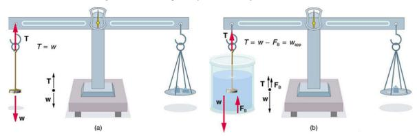
Figure 11.24 (a) A coin is weighed in air. (b) The apparent weight of the coin is determined while it is completely submerged in a fluid of known density. These two measurements are used to calculate the density of the coin.
