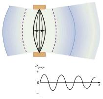
**Figure 17.5** After many vibrations, there are a series of compressions and rarefactions moving out from the string as a sound wave. The graph shows gauge pressure versus distance from the source. Pressures vary only slightly from atmospheric for ordinary sounds.
