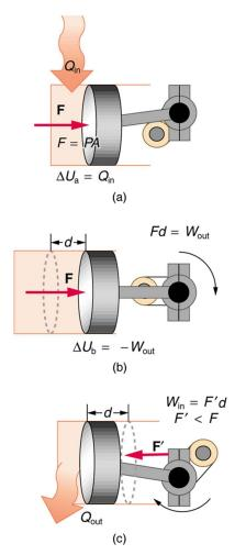
Figure 15.8 (a) Heat transfer to the gas in a cylinder increases the internal energy of the gas, creating higher pressure and temperature. (b) The force exerted on the movable cylinder does work as the gas expands. Gas pressure and temperature decrease when it expands, indicating that the gas's internal energy has been decreased by doing work. (c) Heat transfer to the environment further reduces pressure in the gas so that the piston can be more easily returned to its starting position.
