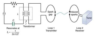
Figure 24.4 The apparatus used by Hertz in 1887 to generate and detect electromagnetic waves. An *RLC* circuit connected to the first loop caused sparks across a gap in the wire loop and generated electromagnetic waves. Sparks across a gap in the second loop located across the laboratory gave evidence that the waves had been received.
