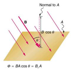
Figure 23.6 Magnetic flux  $\Phi$  is related to the magnetic field and the area over which it exists. The flux  $\Phi = BA \cos \theta$  is related to induction; any change in  $\Phi$  induces an emf.
