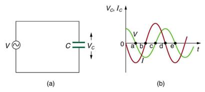
Figure 23.46 (a) An AC voltage source in series with a capacitor *C* having negligible resistance. (b) Graph of current and voltage across the capacitor as functions of time.
