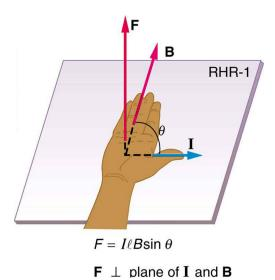
Figure 22.31 The force on a current-carrying wire in a magnetic field is  $F = IlB \sin \theta$ . Its direction is given by RHR-1.
