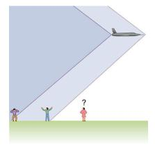
Figure 17.17 Two sonic booms, created by the nose and tail of an aircraft, are observed on the ground after the plane has passed by.
