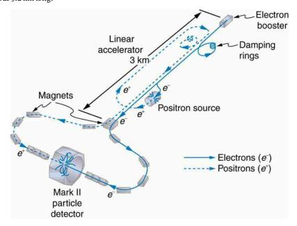
Figure 33.11 The Stanford Linear Accelerator was 3.2 km long and had the capability of colliding electron and positron beams. SLAC was also used to probe nucleons by scattering extremely short wavelength electrons from them. This produced the first convincing evidence of a quark structure inside nucleons in an experiment analogous to those performed by Rutherford long ago.
