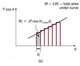
Figure 7.3 (a) A graph of  $F \cos \theta$  vs. d, when  $F \cos \theta$  is constant. The area under the curve represents the work done by the force. (b) A graph of  $F \cos \theta$  vs. d in which the force varies. The work done for each interval is the area of each strip; thus, the total area under the curve equals the total work done.
