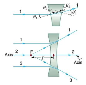
Figure 25.29 Rays of light entering a diverging lens parallel to its axis are diverged, and all appear to originate at its focal point F. The dashed lines are not rays—they indicate the directions from which the rays appear to come. The focal length f of a diverging lens is negative. An expanded view of the path taken by ray 1 shows the perpendiculars and the angles of incidence and refraction at both surfaces.
