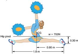
**Figure 9.35** A gymnast performs full split. The center of gravity and the various distances from it are shown.
