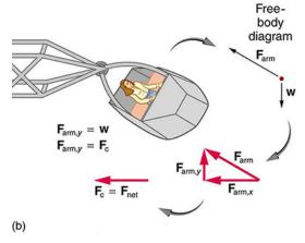
Figure 6.37 (a) NASA centrifuge used to subject trainees to accelerations similar to those experienced in rocket launches and reentries. (credit: NASA) (b) Rider in cage showing how the cage pivots outward during rotation. This allows the total force exerted on the rider by the cage to be along its axis at all times.
