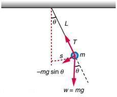
Figure 16.14 A simple pendulum has a small-diameter bob and a string that has a very small mass but is strong enough not to stretch appreciably. The linear displacement from equilibrium is s, the length of the arc. Also shown are the forces on the bob, which result in a net force of  $-mg \sin\theta$  toward the equilibrium position—that is, a restoring force.
