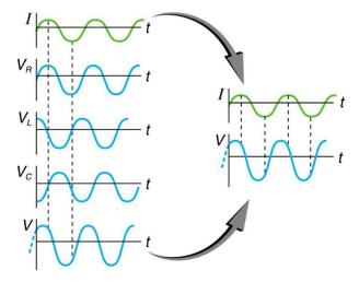
Figure 23.49 This graph shows the relationships of the voltages in an *RLC* circuit to the current. The voltages across the circuit elements add to equal the voltage of the source, which is seen to be out of phase with the current.
