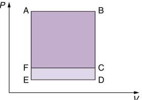
Figure 15.41 The two cyclical processes shown on this PV diagram start with and return the system to the conditions at point A, but they follow different paths and produce different amounts of work.
