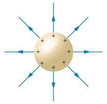
Figure 18.32 The mutual repulsion of excess positive charges on a spherical conductor distributes them uniformly on its surface. The resulting electric field is perpendicular to the surface and zero inside. Outside the conductor, the field is identical to that of a point charge at the center equal to the excess charge.
