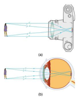
Figure 25.34 Real images can be projected. (a) A real image of the person is projected onto film. (b) The converging nature of the multiple surfaces that make up the eye result in the projection of a real image on the retina.
