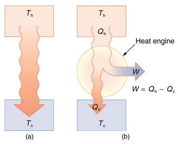
Figure 15.17 (a) Heat transfer occurs spontaneously from a hot object to a cold one, consistent with the second law of thermodynamics. (b) A heat engine, represented here by a circle, uses part of the heat transfer to do work. The hot and cold objects are called the hot and cold reservoirs.  $Q_b$  is the heat transfer out of the hot reservoir. W is the work output, and  $Q_c$  is the heat transfer into the cold reservoir.
