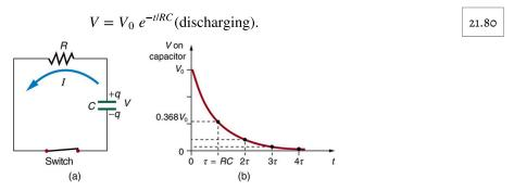
Figure 21.39 (a) Closing the switch discharges the capacitor C through the resistor R. Mutual repulsion of like charges on each plate drives the current. (b) A graph of voltage across the capacitor versus time, with  $V=V_0$  at t=0. The voltage decreases exponentially, falling a fixed fraction of the way to zero in each subsequent time constant  $\tau$ .
