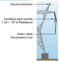
Figure 21.51 High-voltage (240-kV) transmission line carrying  $5.00\times 10^2~{\rm A}$  is hung from a grounded metal transmission tower. The row of ceramic insulators provide  $1.00\times 10^9 \Omega$  of resistance each.
