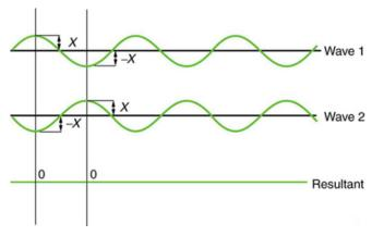
Figure 16.37 Pure destructive interference of two identical waves produces zero amplitude, or complete cancellation.
