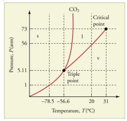
Figure 13.35 The phase diagram for carbon dioxide. The axes are nonlinear, and the graph is not to scale. Dry ice is solid carbon dioxide and has a sublimation temperature of –78.5°C.
