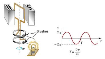
Figure 23.22 The emf of a generator is sent to a light bulb with the system of rings and brushes shown. The graph gives the emf of the generator as a function of time. emf<sub>0</sub> is the peak emf. The period is  $T = 1/f = 2\pi/\omega$ , where f is the frequency. Note that the script E stands for emf.
