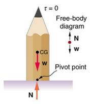
Figure 9.10 This pencil is in the condition of equilibrium. The net force on the pencil is zero and the total torque about any pivot is zero.
