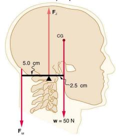
Figure 9.40 The center of mass of the head lies in front of its major point of support, requiring muscle action to hold the head erect. A simplified lever system is shown.
