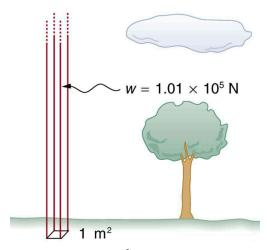
Figure 11.11 Atmospheric pressure at sea level averages  $1.01 \times 10^5$  Pa (equivalent to 1 atm), since the column of air over this  $1 \text{ m}^2$ , extending to the top of the atmosphere, weighs  $1.01 \times 10^5$  N.
