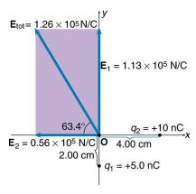
Figure 18.24 The electric fields  $E_1$  and  $E_2$  at the origin O add to  $E_{tot}$ .
