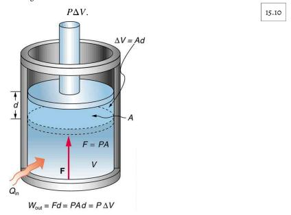
Figure 15.9 An isobaric expansion of a gas requires heat transfer to keep the pressure constant. Since pressure is constant, the work done is  $P\Delta V$ .
