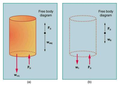
Figure 11.20 (a) An object submerged in a fluid experiences a buoyant force  $F_B$ . If  $F_B$  is greater than the weight of the object, the object will rise. If  $F_B$  is less than the weight of the object, the object will sink. (b) If the object is removed, it is replaced by fluid having weight  $w_{fl}$ . Since this weight is supported by surrounding fluid, the buoyant force must equal the weight of the fluid displaced. That is,  $F_B = w_{fl}$ , a statement of Archimedes' principle.
