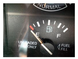
Figure 13.13 Because the gas expands more than the gas tank with increasing temperature, you can't drive as many miles on "empty" in the summer as you can in the winter. (credit: Hector Alejandro, Flickr)
