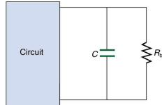
Figure 21.50 A bleeder resistor  $R_{\rm bl}$  discharges the capacitor in this electronic device once it is switched off.
