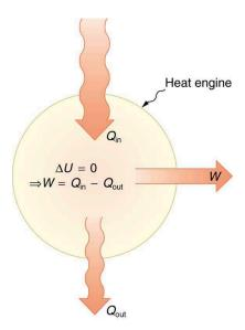
Figure 15.7 Schematic representation of a heat engine, governed, of course, by the first law of thermodynamics. It is impossible to devise a system where  $Q_{\text{out}} = 0$ , that is, in which no heat transfer occurs to the environment.
