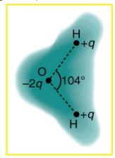
Figure 18.43 Schematic representation of the outer electron cloud of a neutral water molecule. The electrons spend more time near the oxygen than the hydrogens, giving a permanent charge separation as shown. Water is thus a *polar molecule*. It is more easily affected by electrostatic forces than molecules with uniform charge distributions.
