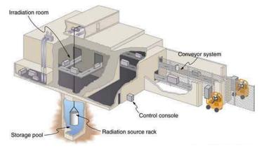
Figure 32.12 A food irradiation plant has a conveyor system to pass items through an intense radiation field behind thick shielding walls. The  $\gamma$  source is lowered into a deep pool of water for safe storage when not in use. Exposure times of up to an hour expose food to doses up to  $10^4$  Gv.
