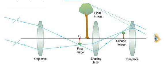
Figure 26.24 This arrangement of three lenses in a telescope produces an upright final image. The first two lenses are far enough apart that the second lens inverts the image of the first one more time. The third lens acts as a magnifier and keeps the image upright and in a location that is easy to view.
