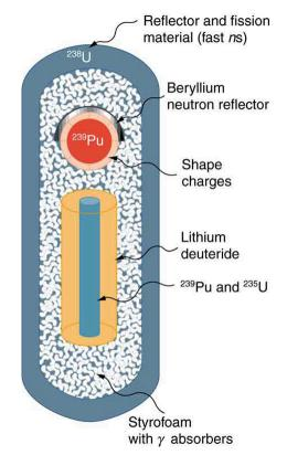
Figure 32.31 This schematic of a fusion bomb (H-bomb) gives some idea of how the  $^{239}$ Pu fission trigger is used to ignite fusion fuel. Neutrons and  $\gamma$  rays transmit energy to the fusion fuel, create tritium from deuterium, and heat and compress the fusion fuel. The outer shell of  $^{238}$ U serves to reflect some neutrons back into the fuel, causing more fusion, and it boosts the energy output by fissioning itself when neutron energies become high enough.
