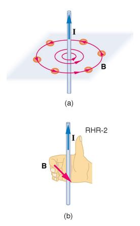
Figure 22.38 (a) Compasses placed near a long straight current-carrying wire indicate that field lines form circular loops centered on the wire. (b) Right hand rule 2 states that, if the right hand thumb points in the direction of the current, the fingers curl in the direction of the field. This rule is consistent with the field mapped for the long straight wire and is valid for any current segment.
