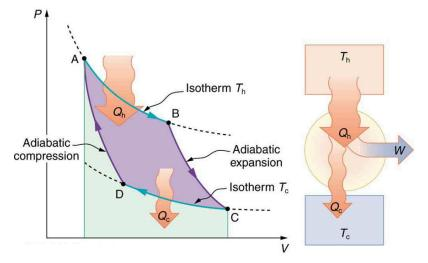
Figure 15.22 PV diagram for a Carnot cycle, employing only reversible isothermal and adiabatic processes. Heat transfer  $Q_h$  occurs into the working substance during the isothermal path AB, which takes place at constant temperature  $T_h$ . Heat transfer  $Q_c$  occurs out of the working substance during the isothermal path CD, which takes place at constant temperature  $T_c$ . The net work output W equals the area
