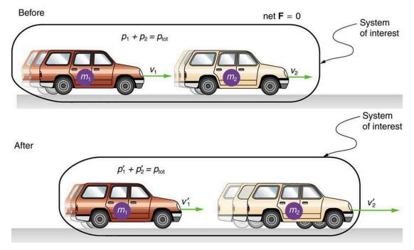
Figure 8.3 A car of mass  $m_1$  moving with a velocity of  $v_1$  bumps into another car of mass  $m_2$  and velocity  $v_2$  that it is following. As a result, the first car slows down to a velocity of  $v'_1$  and the second speeds up to a velocity of  $v'_2$ . The momentum of each car is changed, but the total momentum  $p_{\text{tot}}$  of the two cars is the same before and after the collision (if you assume friction is negligible).
