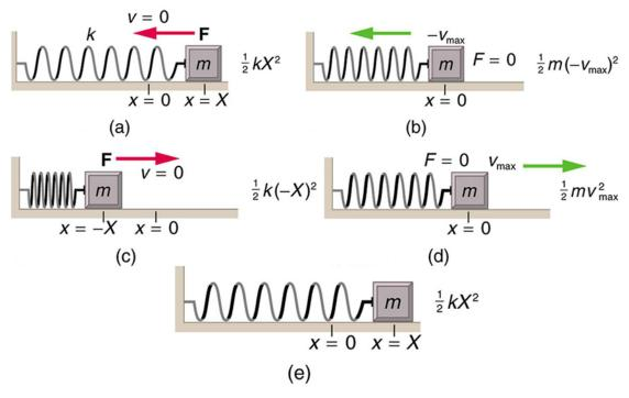
Figure 16.16 The transformation of energy in simple harmonic motion is illustrated for an object attached to a spring on a frictionless surface.
