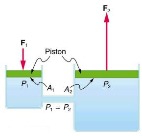
Figure 11.12 A typical hydraulic system with two fluid-filled cylinders, capped with pistons and connected by a tube called a hydraulic line. A downward force  $\mathbf{F}_1$  on the left piston creates a pressure that is transmitted undiminished to all parts of the enclosed fluid. This results in an upward force  $\mathbf{F}_2$  on the right piston that is larger than  $\mathbf{F}_1$  because the right piston has a larger area.
