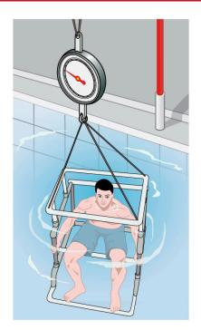
Figure 11.23 Subject in a "fat tank," where he is weighed while completely submerged as part of a body density determination. The subject must completely empty his lungs and hold a metal weight in order to sink. Corrections are made for the residual air in his lungs (measured separately) and the metal weight. His corrected submerged weight, his weight in air, and pinch tests of strategic fatty areas are used to calculate his percent body fat.
