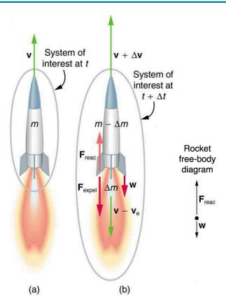
Figure 8.13 (a) This rocket has a mass m and an upward velocity v. The net external force on the system is -mg, if air resistance is neglected. (b) A time  $\Delta t$  later the system has two main parts, the ejected gas and the remainder of the rocket. The reaction force on the rocket is what overcomes the gravitational force and accelerates it upward.
