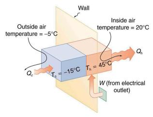
Figure 15.30 Heat transfer from the outside to the inside, along with work done to run the pump, takes place in the heat pump of the example above. Note that the cold temperature produced by the heat pump is lower than the outside temperature, so that heat transfer into the working fluid occurs. The pump's compressor produces a temperature greater than the indoor temperature in order for heat transfer into the house to occur.
