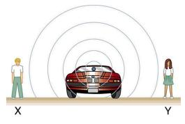
Figure 17.13 Sounds emitted by a source spread out in spherical waves. Because the source, observers, and air are stationary, the wavelength and frequency are the same in all directions and to all observers.
