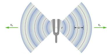
Figure 17.8 A sound wave emanates from a source vibrating at a frequency f, propagates at  $v_w$ , and has a wavelength  $\lambda$ .
