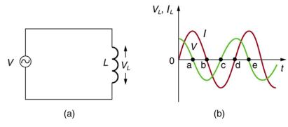
Figure 23.45 (a) An AC voltage source in series with an inductor having negligible resistance. (b) Graph of current and voltage across the inductor as functions of time.
