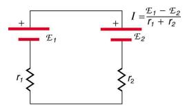
Figure 21.17 These two voltage sources are connected in series with their emfs in opposition. Current flows in the direction of the greater emf and is limited to  $I = \frac{(\text{emf}_1 - \text{emf}_2)}{r_1 + r_2}$  by the sum of the internal resistances. (Note that each emf is represented by script E in the figure.) A battery charger connected to a battery is an example of such a connection. The charger must have a larger emf than the battery to reverse current through it.
