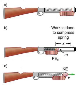
Figure 16.7 (a) In this image of the gun, the spring is uncompressed before being cocked. (b) The spring has been compressed a distance x, and the projectile is in place. (c) When released, the spring converts elastic potential energy  $PE_{el}$  into kinetic energy.
