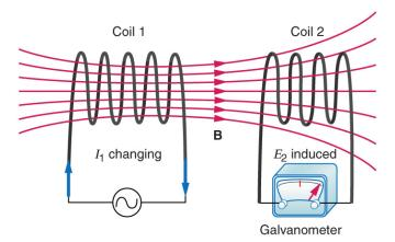
Figure 23.39 These coils can induce emfs in one another like an inefficient transformer. Their mutual inductance M indicates the effectiveness of the coupling between them. Here a change in current in coil 1 is seen to induce an emf in coil 2. (Note that " $E_2$  induced" represents the induced emf in coil 2.)
