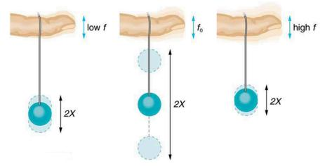
Figure 16.26 The paddle ball on its rubber band moves in response to the finger supporting it. If the finger moves with the natural frequency  $f_0$  of the ball on the rubber band, then a resonance is achieved, and the amplitude of the ball's oscillations increases dramatically. At higher and lower driving frequencies, energy is transferred to the ball less efficiently, and it responds with lower-amplitude oscillations.
