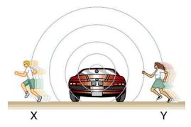
Figure 17.15 The same effect is produced when the observers move relative to the source. Motion toward the source increases frequency as the observer on the right passes through more wave crests than she would if stationary. Motion away from the source decreases frequency as the observer on the left passes through fewer wave crests than he would if stationary.
