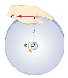
Figure 10.17 A large grindstone is given a spin by a person grasping its outer edge.
