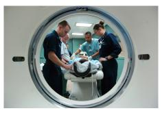
Figure 30.27 A patient being positioned in a CT scanner aboard the hospital ship USNS Mercy. The CT scanner passes x rays through slices of the patient's body (or body part) over a range of directions. The relative absorption of the x rays along different directions is computer analyzed to produce highly detailed images. Three-dimensional information can be obtained from multiple slices. (credit: Rebecca Moat, U.S. Navy)
