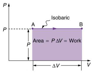
**Figure 15.10** A graph of pressure versus volume for a constant-pressure, or isobaric, process, such as the one shown in <u>Figure 15.9</u>. The area under the curve equals the work done by the gas, since  $W = P\Delta V$ .
