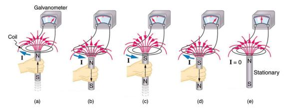
Figure 23.4 Movement of a magnet relative to a coil produces emfs as shown. The same emfs are produced if the coil is moved relative to the magnet. The greater the speed, the greater the magnitude of the emf, and the emf is zero when there is no motion.
