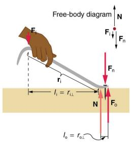
Figure 9.22 A nail puller is a lever with a large mechanical advantage. The external forces on the nail puller are represented by solid arrows. The force that the nail puller applies to the nail ( $\mathbf{F}_{o}$ ) is not a force on the nail puller. The reaction force the nail exerts back on the puller ( $\mathbf{F}_{n}$ ) is an external force and is equal and opposite to  $\mathbf{F}_{o}$ . The perpendicular lever arms of the input and output forces are  $l_{i}$  and  $l_{o}$ .
