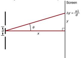
Figure 27.57 The distance between adjacent fringes is  $\Delta y = x \lambda / d$ , assuming the slit separation d is large compared with  $\lambda$ .
