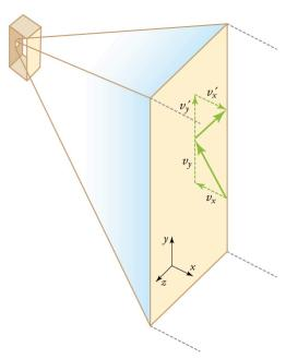
Figure 13.21 Gas in a box exerts an outward pressure on its walls. A molecule colliding with a rigid wall has the direction of its velocity and momentum in the *x*-direction reversed. This direction is perpendicular to the wall. The components of its velocity momentum in the *y*- and *z*-directions are not changed, which means there is no force parallel to the wall.
