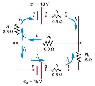
Figure 21.25 This circuit is similar to that in Figure 21.21, but the resistances and emfs are specified. (Each emf is denoted by script E.) The currents in each branch are labeled and assumed to move in the directions shown. This example uses Kirchhoff's rules to find the currents.
