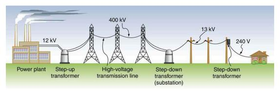
Figure 23.27 Transformers change voltages at several points in a power distribution system. Electric power is usually generated at greater than 10 kV, and transmitted long distances at voltages over 200 kV—sometimes as great as 700 kV—to limit energy losses. Local power distribution to neighborhoods or industries goes through a substation and is sent short distances at voltages ranging from 5 to 13 kV. This is reduced to 120, 240, or 480 V for safety at the individual user site.
