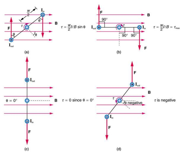
Figure 22.35 Top views of a current-carrying loop in a magnetic field. (a) The equation for torque is derived using this view. Note that the perpendicular to the loop makes an angle  $\theta$  with the field that is the same as the angle between w/2 and  $\mathbf{F}$ . (b) The maximum torque occurs when  $\theta$  is a right angle and  $\sin\theta=1$ . (c) Zero (minimum) torque occurs when  $\theta$  is zero and  $\sin\theta=0$ . (d) The torque reverses once the loop rotates past  $\theta=0$ .
