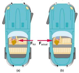
Figure 6.15 (a) The car driver feels herself forced to the left relative to the car when she makes a right turn. This is a fictitious force arising from the use of the car as a frame of reference. (b) In the Earth's frame of reference, the driver moves in a straight line, obeying Newton's first law, and the car moves to the right. There is no real force to the left on the driver relative to Earth. There is a real force to the right on the car to make it turn.
