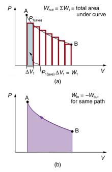
**Figure 15.11** (a) A *PV* diagram in which pressure varies as well as volume. The work done for each interval is its average pressure times the change in volume, or the area under the curve over that interval. Thus the total area under the curve equals the total work done. (b) Work must be done on the system to follow the reverse path. This is interpreted as a negative area under the curve.
