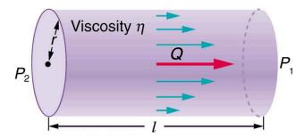
Figure 12.14 Poiseuille's law applies to laminar flow of an incompressible fluid of viscosity  $\eta$  through a tube of length l and radius r. The direction of flow is from greater to lower pressure. Flow rate Q is directly proportional to the pressure difference  $P_2 - P_1$ , and inversely proportional to the length l of the tube and viscosity  $\eta$  of the fluid. Flow rate increases with  $r^4$ , the fourth power of the radius.
