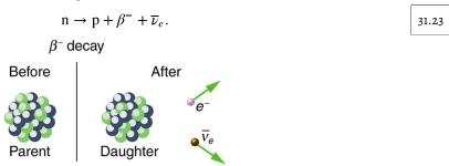
Figure 31.19 In  $\beta^-$  decay, the parent nucleus emits an electron and an antineutrino. The daughter nucleus has one more proton and one less neutron than its parent. Neutrinos interact so weakly that they are almost never directly observed, but they play a fundamental role in
