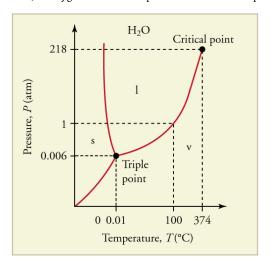
**Figure 13.28** The phase diagram (*PT* graph) for water. Note that the axes are nonlinear and the graph is not to scale. This graph is simplified—there are several other exotic phases of ice at higher pressures.
