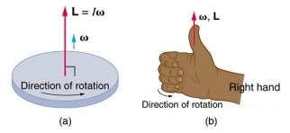
Figure 10.28 Figure (a) shows a disk is rotating counterclockwise when viewed from above. Figure (b) shows the right-hand rule. The direction of angular velocity  $\omega$  size and angular momentum L are defined to be the direction in which the thumb of your right hand points when you curl your fingers in the direction of the disk's rotation as shown.
