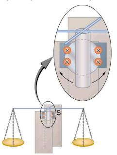
Figure 23.16 Magnetic damping of this sensitive balance slows its oscillations. Since Faraday's law of induction gives the greatest effect for the most rapid change, damping is greatest for large oscillations and goes to zero as the motion stops.
