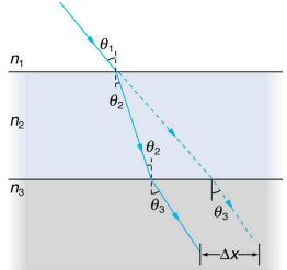
Figure 25.54 A ray of light passes from one medium to a third by traveling through a second. The final direction is the same as if the second medium were not present, but the ray is displaced by  $\Delta x$  (shown exaggerated).
