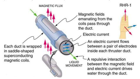
Figure 22.33 An MHD propulsion system in a nuclear submarine could produce significantly less turbulence than propellers and allow it to run more silently. The development of a silent drive submarine was dramatized in the book and the film *The Hunt for Red October*.
