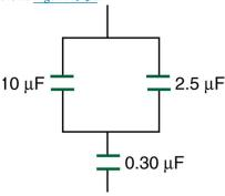
**Figure 19.32** A combination of series and parallel connections of capacitors.
