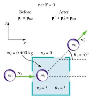
Figure 8.12 A collision taking place in a dark room is explored in Example 8.7. The incoming object  $m_1$  is scattered by an initially stationary object. Only the stationary object's mass  $m_2$  is known. By measuring the angle and speed at which  $m_1$  emerges from the room, it is possible to calculate the magnitude and direction of the initially stationary object's velocity after the collision.
