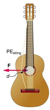
Figure 7.11 Work is done to deform the guitar string, giving it potential energy. When released, the potential energy is converted to kinetic energy and back to potential as the string oscillates back and forth. A very small fraction is dissipated as sound energy, slowly removing energy from the string.
