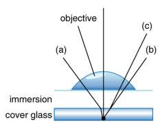
Figure 26.19 Light rays from a specimen entering the objective. Paths for immersion medium of air (a), water (b) (n = 1.33), and oil (c) (n = 1.51) are shown. The water and oil immersions allow more rays to enter the objective, increasing the resolution.
