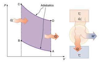
Figure 15.20 This Otto cycle produces a greater work output than the one in Figure 15.19, because the starting temperature of path CD is higher and the starting temperature of path AB is lower. The area inside the loop is greater, corresponding to greater net work output.
