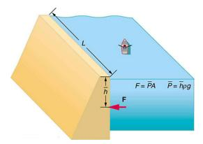
Figure 11.10 The dam must withstand the force exerted against it by the water it retains. This force is small compared with the weight of the water behind the dam.
