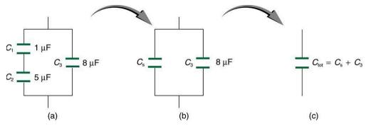
Figure 19.22 (a) This circuit contains both series and parallel connections of capacitors. See Example 19.10 for the calculation of the
