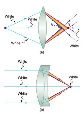
Figure 26.28 (a) Chromatic aberration is caused by the dependence of a lens's index of refraction on color (wavelength). The lens is more powerful for violet (V) than for red (R), producing images with different locations and magnifications. (b) Multiple-lens systems can partially correct chromatic aberrations, but they may require lenses of different materials and add to the expense of optical systems such as cameras.
