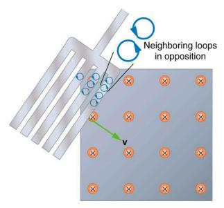
Figure 23.15 Eddy currents induced in a slotted metal plate entering a magnetic field form small loops, and the forces on them tend to cancel, thereby making magnetic drag almost zero.
