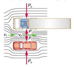
Figure 12.4 An overhead view of a car passing a truck on a highway. Air passing between the vehicles flows in a narrower channel and must increase its speed ( $v_2$  is greater than  $v_1$ ), causing the pressure between them to drop ( $P_i$  is less than  $P_o$ ). Greater pressure on the outside pushes the car and truck together.
