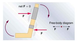
Figure 9.5 The same forces are applied at other points and the stick rotates—in fact, it experiences an accelerated rotation. Here net  $\mathbf{F} = 0$  but the system is *not* at equilibrium. Hence, the net  $\mathbf{F} = 0$  is a necessary—but not sufficient—condition for achieving equilibrium.
