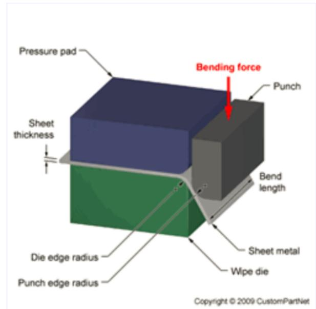
The amount of force required to bend a piece of material into a new permanent shape. The bending force must create enough stress in the material to exceed the yield strength, allowing the material to plastically deform.
