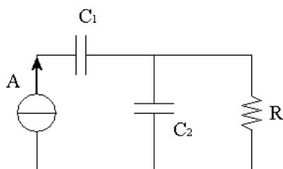
$$\begin{aligned} C_1 &= 0,0003 \text{ F} \\ C_2 &= 0,0005 \text{ F} \\ R &= 20 \, \Omega \\ E &= 80 \text{ V} \\ f &= 50 \text{ Hz} \end{aligned}$$
