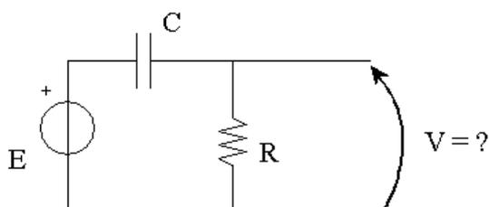
$$\begin{aligned} C &= 0,0003 \text{ F} \\ R &= 10 \, \Omega \\ E &= 60 \text{ V} \\ \omega &= 314 \text{ rad/s} \end{aligned}$$
