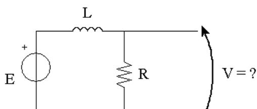
$$\begin{aligned} L &= 0,03 \text{ H} \\ R &= 20 \, \Omega \\ E &= 100 \text{ V} \\ \omega &= 314 \text{ rad/s} \end{aligned}$$
