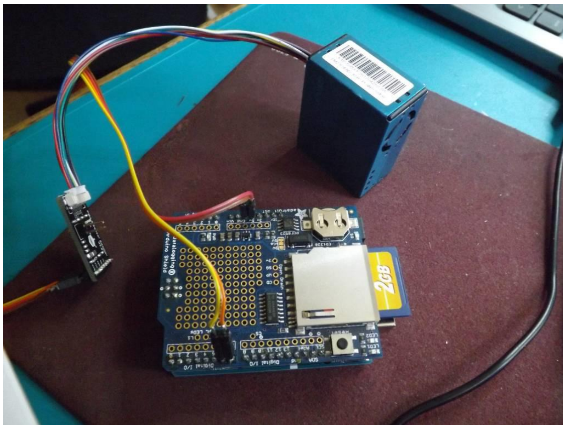
Fig. 7: Plantower PMS5003 device connected to an Arduino based datalogger
