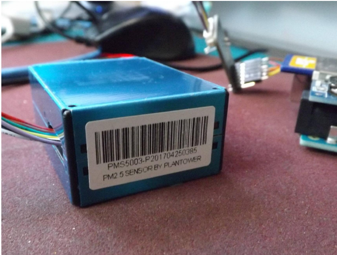
Fig. 8: The PMS5003 with attached product sticker designating it as PM2.5 sensor
