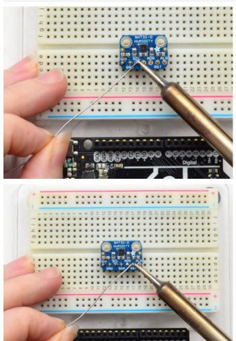
And Solder! Be sure to solder all pins for reliable electrical contact.
