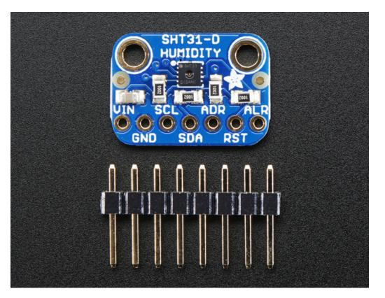
Such a lovely chip - so we spun up a breakout board with the SHT31-D and some supporting circuitry such as pullup resistors and capacitors. Each order comes with one fully assembled and tested PCB breakout and a small piece of header. You'll need to solder the header onto the PCB but it's fairly easy and takes only a few minutes even for a beginner.
