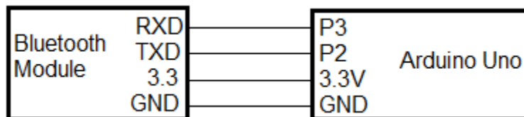
Figure 1. Bluetooth Module – Arduino Uno Connectivity
