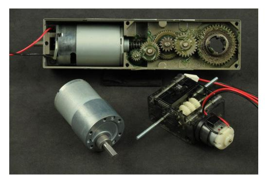
Adding a gear-train to the output of any motor will reduce the speed, while simultaneously increasing torque. Gearing can be added to any type of motor. There is no need to waste time designing a geartrain and sourcing all the parts. Chances are, there is a gearmotor solution that you can drop right into your design.
