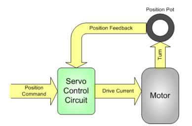
The technical definition of a "Servo Motor" is a motor which employs negative feedback to control motor speed and/or position. Servo feedback senses the difference between the actual and desired speed or position so that the controller can adjust the output to correct the 'error'. Servo control systems are capable of very precise motion control. They are used in everything from high-speed CNC machines to positioning motors for telescope mirrors.
