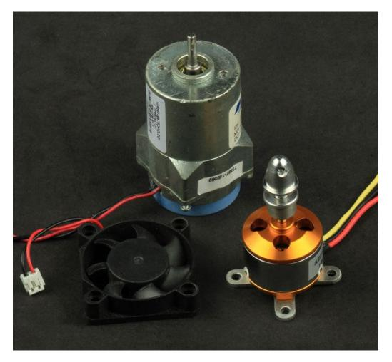
Brushless DC (BLDC) Motors are mechanically simpler than brushed motors. They replace the brushes and associated sparks and noise with electronic commutation to silently switch the current flow to drive the motor. These quiet motors can be found in computer fans and disk drives, as well as in quadcopters, electric vehicles and high-precision servomechanisms.
