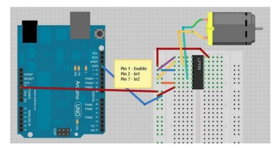
The three pins of L293D that we are interested in are Pin 1 (Enable), Pin 2 (In1) and Pin 7 (In2). These are attached to either 5V or GND using the purple, yellow and orange jumper wires.
