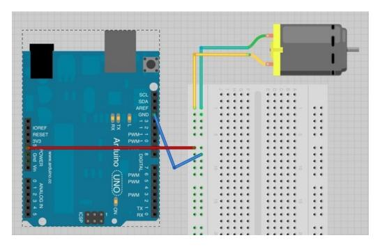
Note which way the motor is spinning. You can do this by pinching the motor shaft between your fingers. Swap over the motor leads so that the motor lead that was going to +5V now goes to GND and vice-versa. The motor will turn in the opposite direction.
