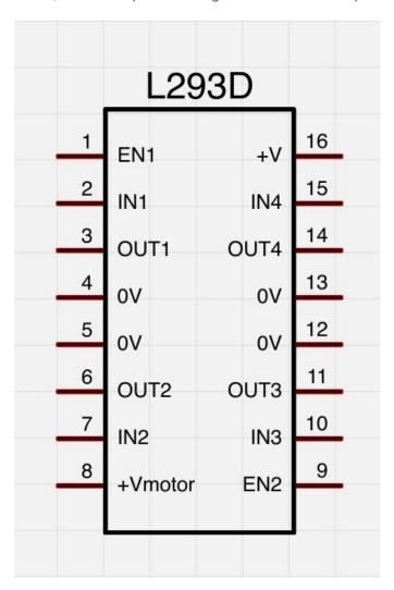
A second motor would be attached between OUT3 and OUT4. You will also need three more control pins.
