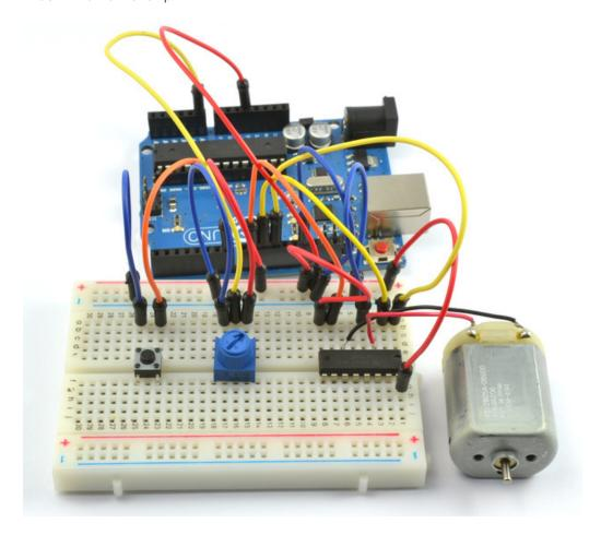
The project uses a pot to control the speed of the motor and a push button to control the direction.
