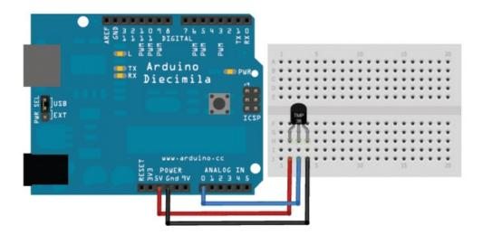
Remember that you can use anywhere between 2.7V and 5.5V as the power supply. For this example I'm showing it with a 5V supply but note that you can use this with a 3.3v supply just as easily. No matter what supply you use, the analog voltage reading will range from about OV (ground) to about 1.75V.
