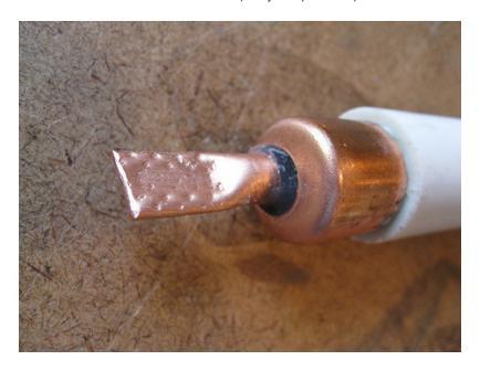
How to waterproof a LM35 sensor for use in a Remotely Operated Vehicle (robot submarine)(https://adafru.it/aKM)
