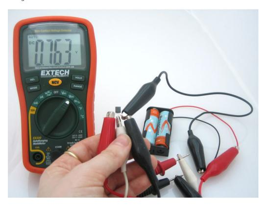
The sensor is indicating that the temperature is 26.3°C also known as 79.3°F
