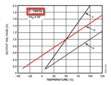
Figure 6. Output Voltage vs. Temperature
