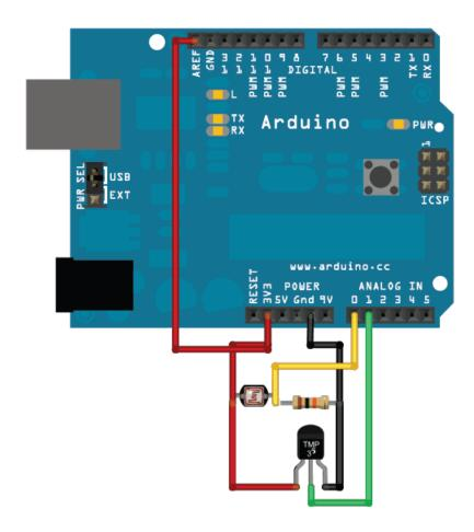
To use the 3.3v pin as your analog reference, don't forget to specify "analogReference(EXTERNAL)" in your setup as in the code below:
