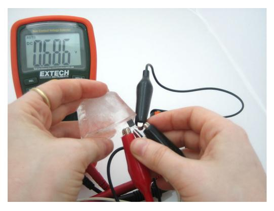
I pressed an ice-cube against the sensor, to bring the temperature down to  $18.6^{\circ}\text{C}/65.5^{\circ}\text{F}$
